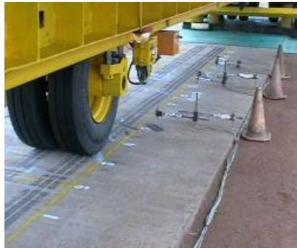
Photo 2 - HVS testing done by GAUTRANS
