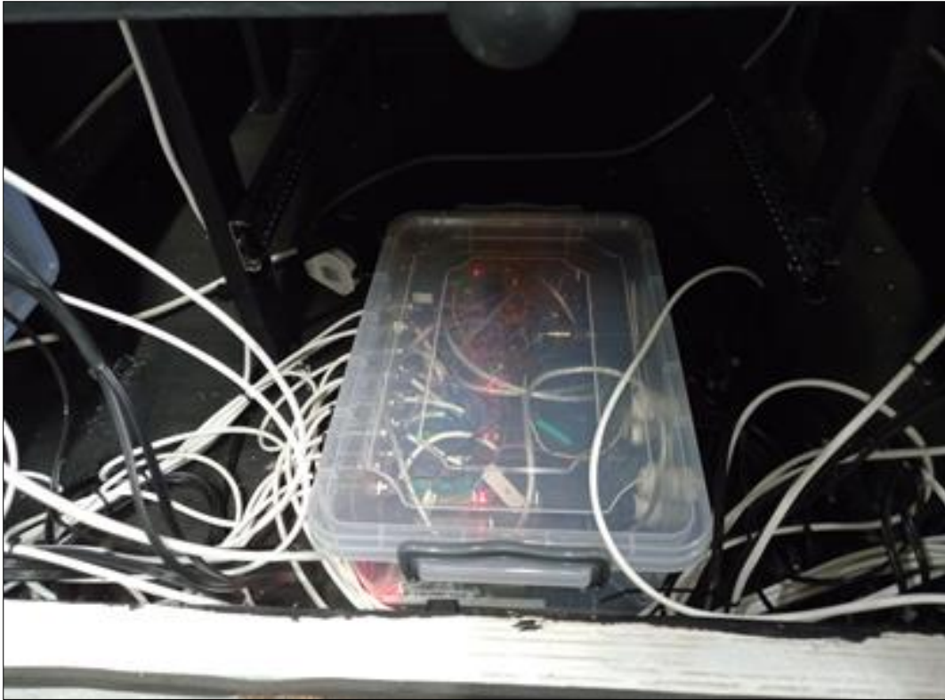
Figure 8: An Arduino microcontroller and associated recording and relay hardware enclosed in a Tupperware to prevent any undesirable contact, but air circulation is provided by the fitted air-conditioner in Fig. 5 above.
