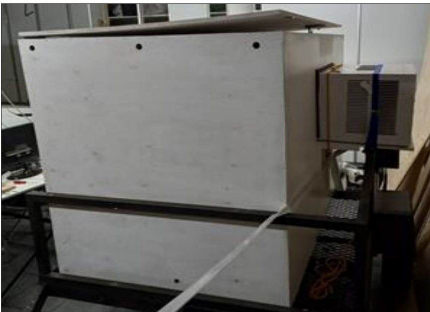
Figure 5: Incubator unit loaded on a trailer for transportation and fitted with an air-conditioner.
