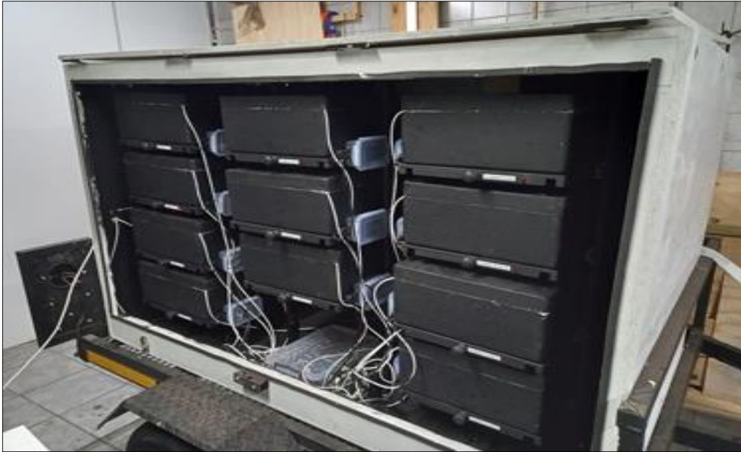
Figure 6: Incubator boxes (from left to right columns: 31\pm 3 °C, 31\pm 6 °C, and 31 °C). Incubator box at bottom centre was removed at the time the picture was taken.
