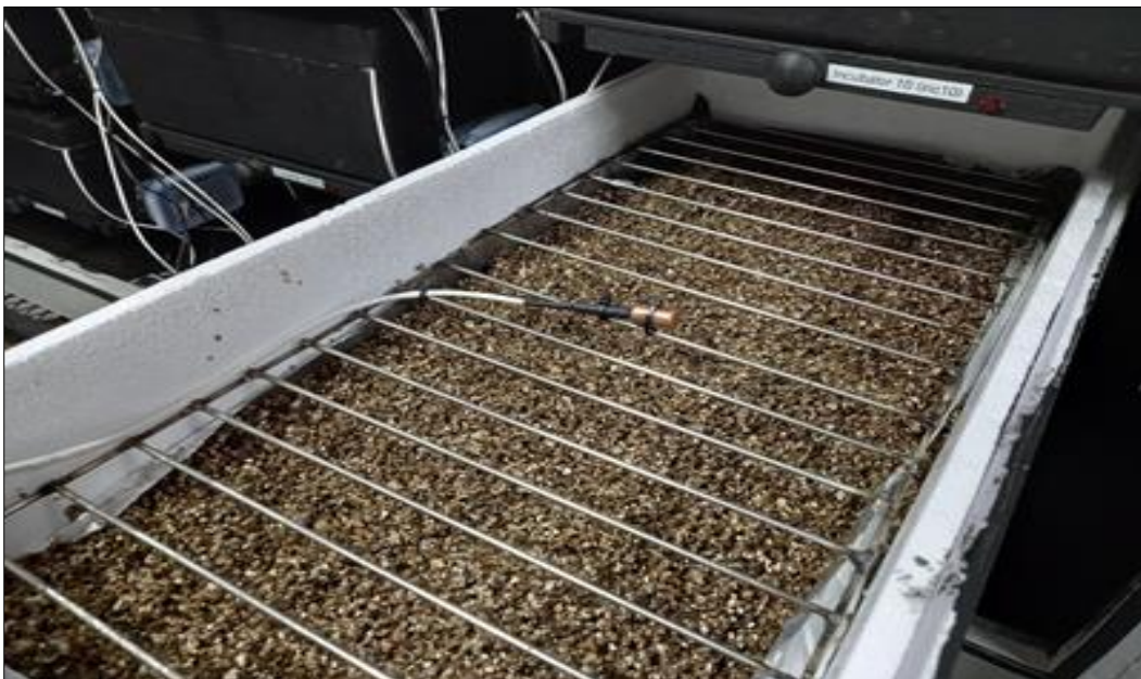
Figure 7: An opened incubator box containing a heating pad, overlaid with moist vermiculite. A temperature sensor is attached to the wire rack.
