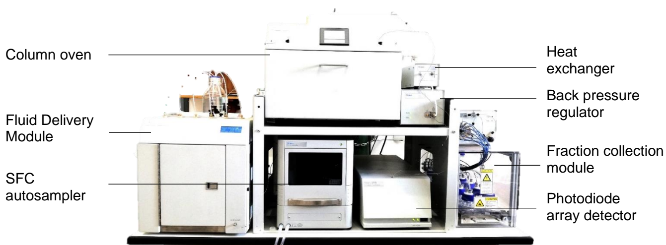
Figure 3.1 Illustration of the Investigator SFC system used to fractionate the crude extract.
