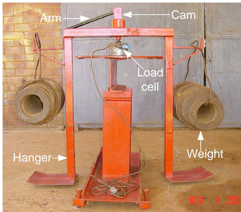
**Figure 4.12:** Calibrating load a cells in compression using a specially designed hanger
