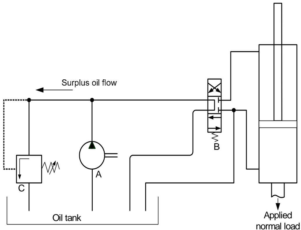
**Figure 4.9:** The special hydraulic circuit for maintaining a constant normal load for the soil shear and frictional shear strength measurement apparatus during sinkage (A – engine driven pump; B – directional control valve; C – flow and pressure control valve with surplus oil back to tank; D – double acting hydraulic cylinder)
