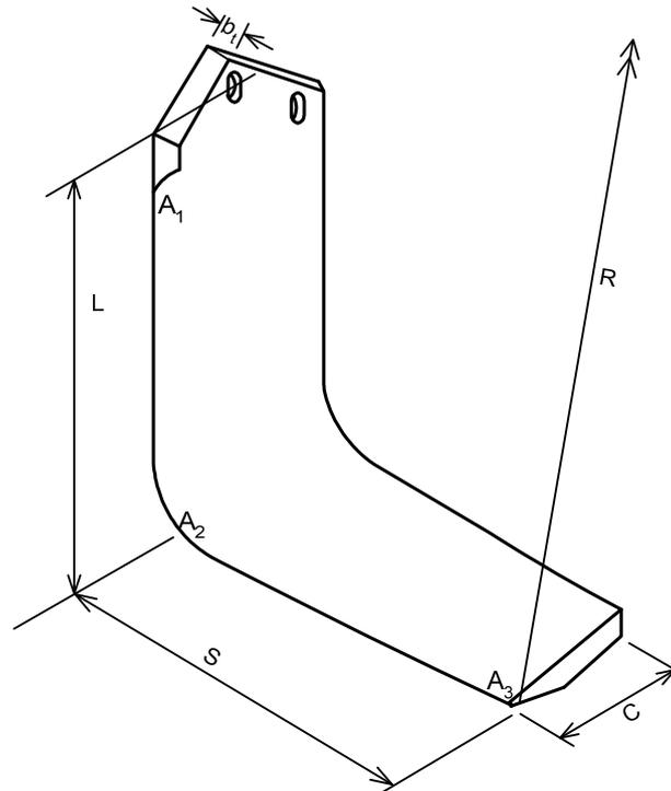
**Figure 3.9:** Line drawing of the standard ‘L-shaped’ blade ( $C$  – chord of the blade, 80 mm at tip and 100 mm at the L–S intersection;  $L$  – vertical section (stem or leg), 100 mm;  $S$  – horizontal section (span), 130 mm;  $b_t$  – thickness of the blade, 7 mm;  $R$  – radius of the rotor, 500 mm;  $\overline{A_1A_2}$  – cutting edge of the leg;  $\overline{A_2A_3}$  – leading edge of the leg)
