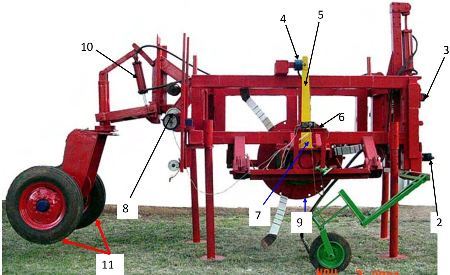
**Figure 4.2:** The fabricated experimental deep rotavators showing some of the key functional components (1- left link force transducer (hidden); 2 – Right lower link force transducer; 3 – top link force transducer; 4 – torque load cell; 5 – torque arm; 6 – magnetic pick-up (hidden); 7 - cable-extension displacement potentiometer; 8 – integrated optical transducer; 9 – hydraulic motor (partly hidden); 10 – double acting cylinder; 11 – swivel wheels)
