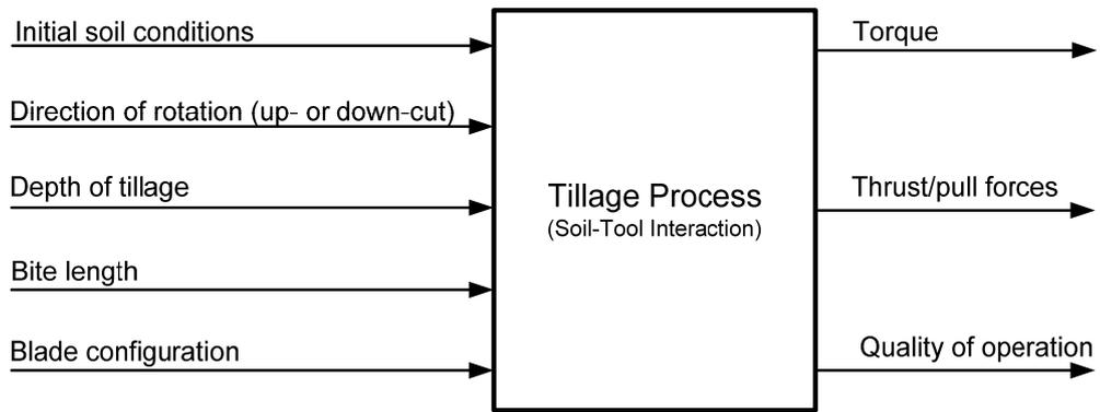
**Figure 1.2:** Proposed block diagram for the rotavator tillage process model
