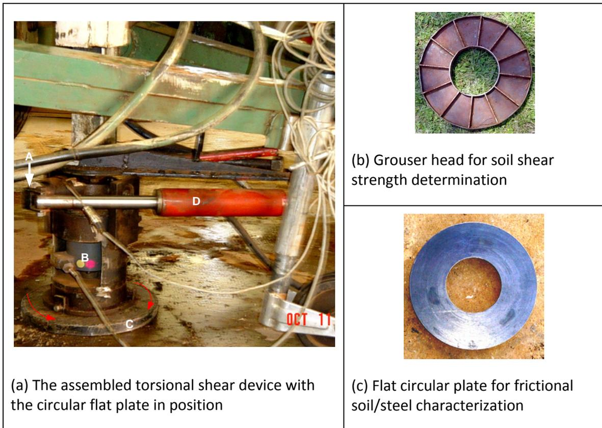
**Figure 4.8:** The fabricated torsional shearing device for determination of soil shear strength and soil-steel frictional parameters (A – torque arm; B –normal/vertical load measuring load-cell; C – grouser head; D – double acting hydraulic cylinder)
