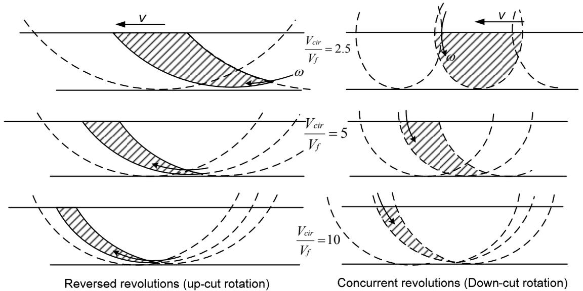
**Figure 3.3:** Shapes of slices for down-cut and up-cut rotation as a function of the ratio of the peripheral speed to forward speed.  $R\omega/V_f = \lambda$ . Number of blades operating in one plane  $z = 3$  (Bernacki *et al.*, 1972)
