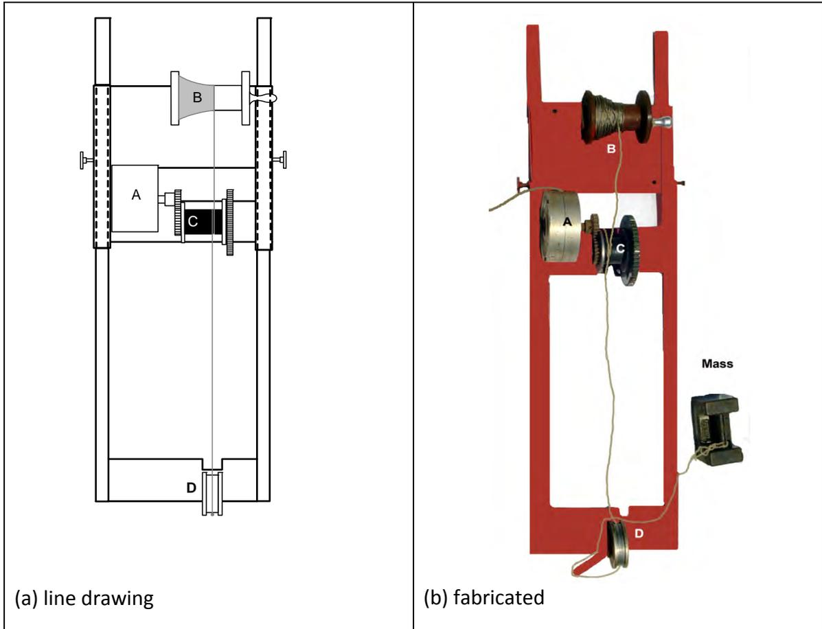
**Figure 4.6:** The assembled ground distance measurement system showing its various components ( A – gearing mechanism with an enclosed integrated optical sensor; B – wire rope wound on a braked drum ; C – rubberised surface on a geared wheel for driving A ; D – wire rope guide)
