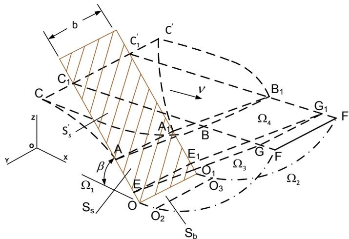
**Figure 2.9:** Failure zone of the Zeng and Yao model (Zeng & Yao, 1992)
