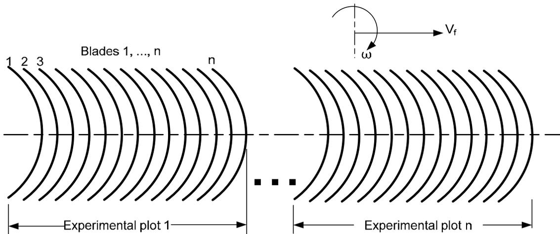
**Figure 5.2:** Illustrations of the cutting paths by individual blades within experimental blocks for experimental plots 1 ... n.
