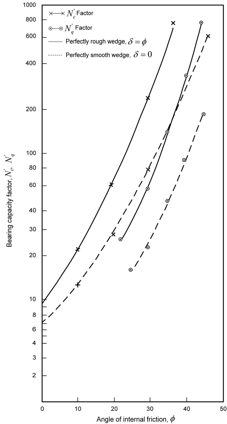
**Figure 3.20:** Relationship between bearing capacity factors and angle of internal friction for deep wedge shaped footing with included tip angle of  $90^\circ$  (Thakur & Godwin, 1989 after Meyerhof, 1951)
