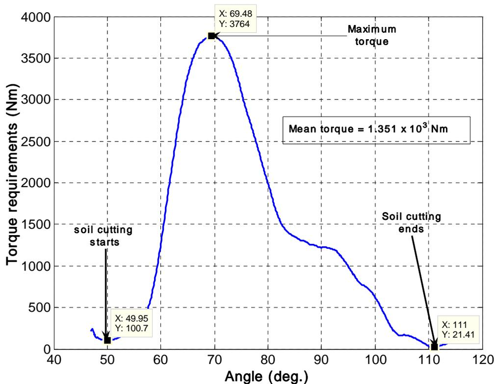
**Figure 6.4:** Typical variation of torque requirements with rotational angle for a single blade between the start and end of soil cutting process [*X*-value = angle turned through by the rotavator blade from the horizontal position; *Y*-value = torque requirement value at position *X*]
