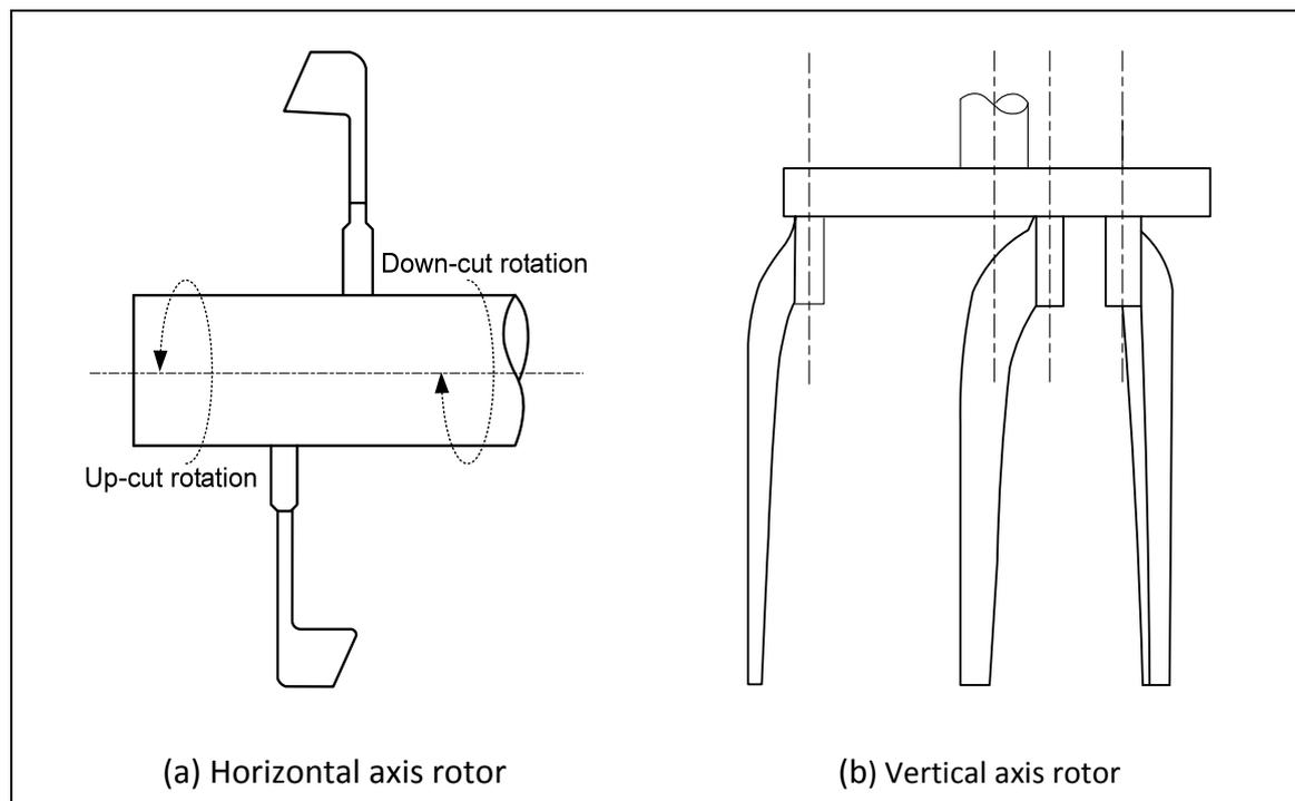
**Figure 1.1:** Illustrations of horizontal and vertical axis rotavators (Bernacki *et al.*, 1972)
