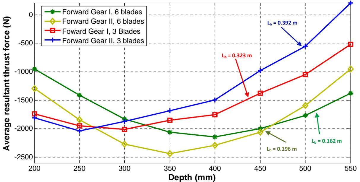
**Figure 6.8:** Variation of the resultant horizontal thrust forces generated at different tillage depths and different bite lengths at a constant soil condition (soil water content of 13.97 %)
