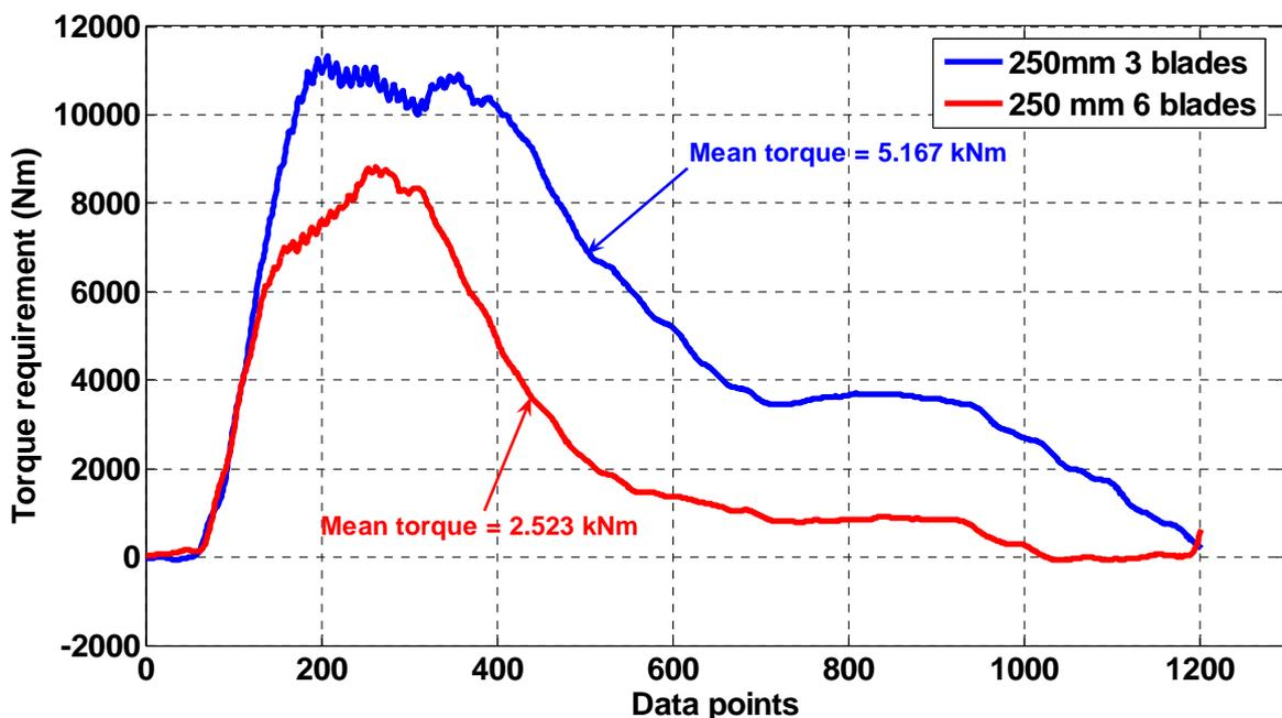
**Figure 6.7:** Effect of bite length on torque requirements
