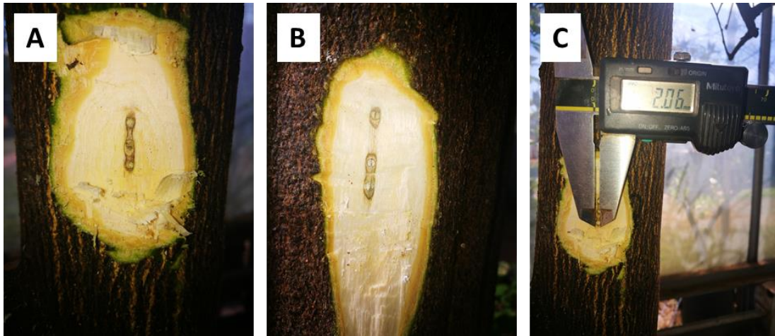
Figure 3-11 Wounding response in 'Midnight' Valencias after HR probe installations (A) and for the CHP probe installations (B), measurement of the wound width with a vernier callipers (C)
