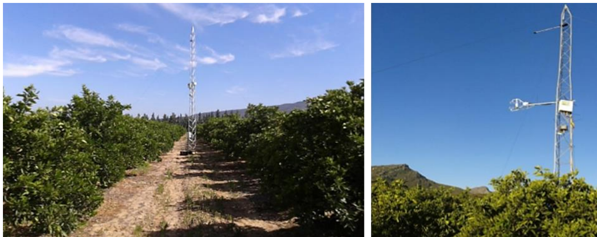
Figure 4-2 Lattice mast in the 'Washington' navels orchard showing position of eddy covariance sensors
