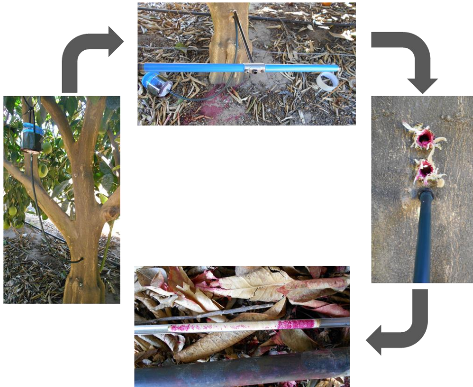
Figure 4-7 Schematic outlay of the process for determining the sapwood depth
