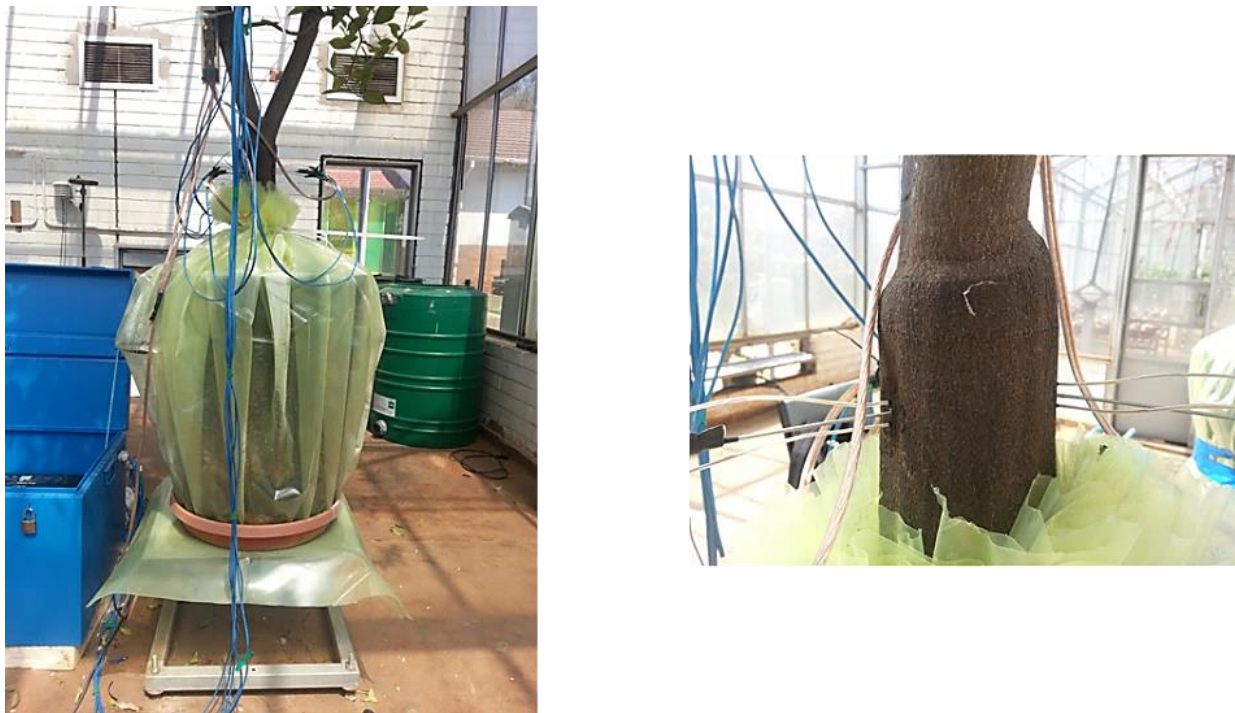
Figure 3-6 Placement of the trees on the weighing lysimeters and probe installation
