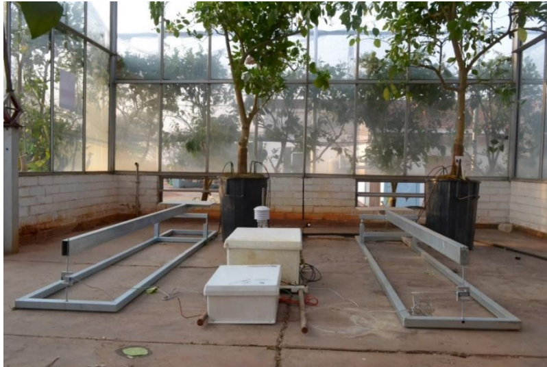
Figure 3-1 Cantilever weighing lysimeters for checking the calibration of sap flow sensors
