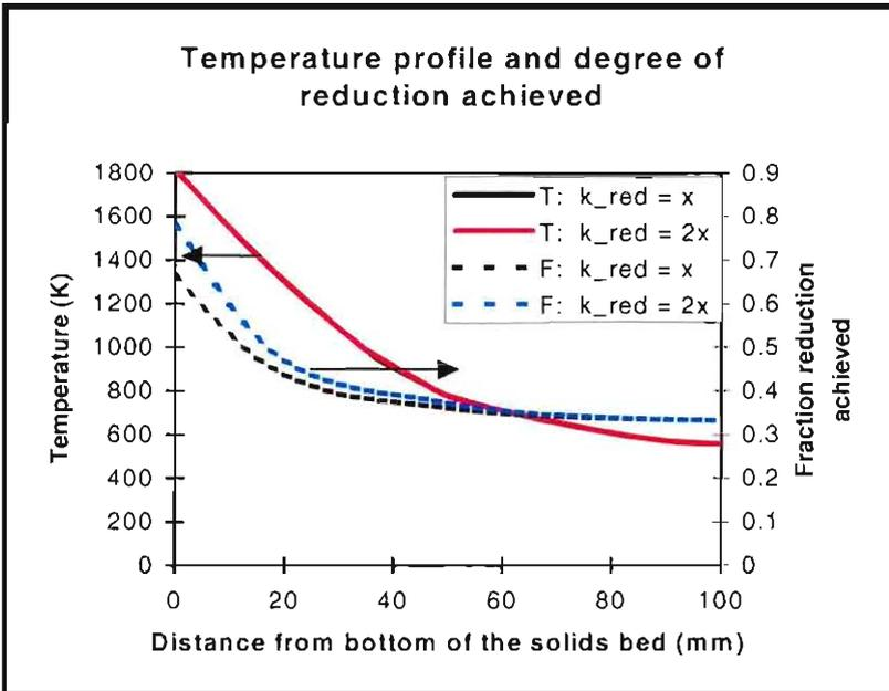
**Figure E 1:** Theoretical profiles of temperature and fraction reduction achieved through a 100mm high solids bed, for a production rate of  $30\text{kg/m}^2/\text{h}$ , when doubling the rate constant for the reduction reaction.
