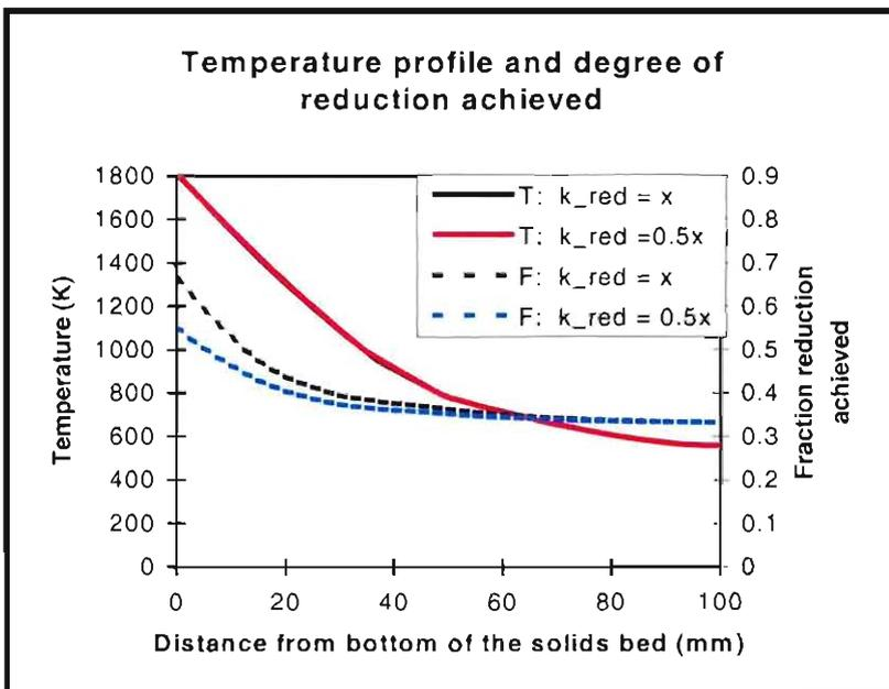
**Figure E 2:** Theoretical profiles of temperature and fraction reduction achieved through a 100mm high solids bed, for a production rate of  $30\text{kg/m}^2/\text{h}$ , when halving the rate constant for the reduction reaction.
