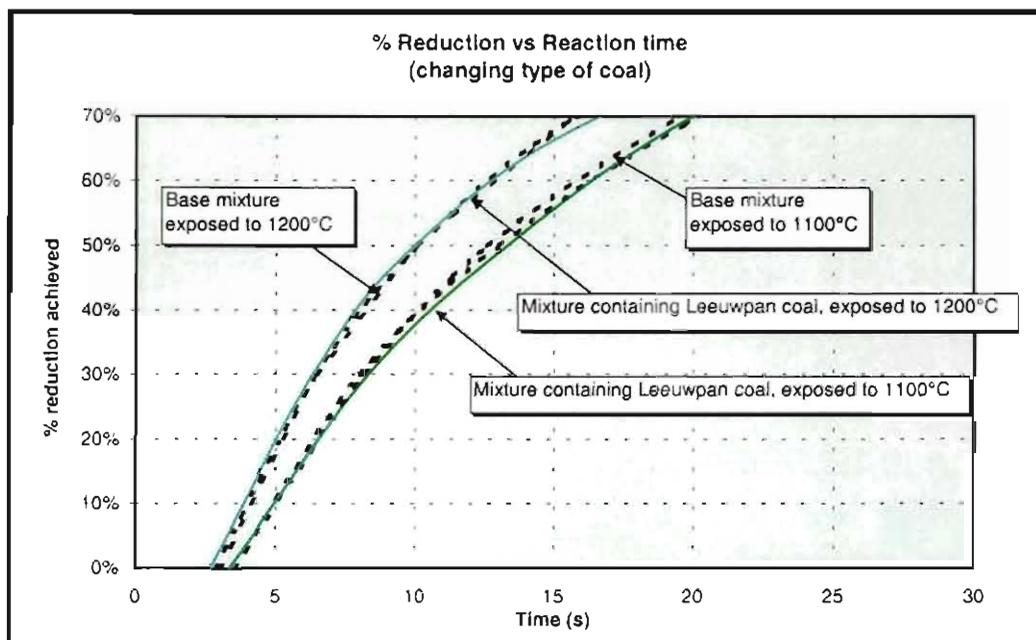
**Figure C 11:** Reduction rate of base mixture and a mixture containing Leeuwan coal exposed to 1100°C and 1200°C.
