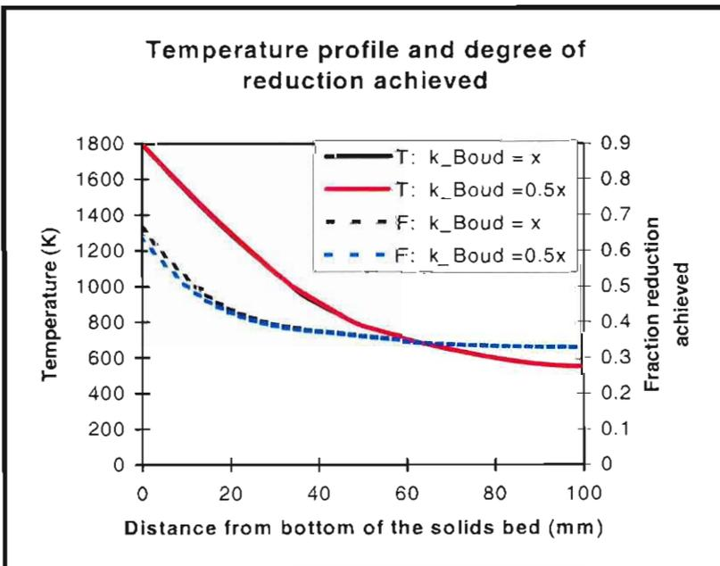
**Figure E 4:** Theoretical profiles of temperature and fraction reduction achieved through a 100mm high solids bed, for a production rate of  $30\text{kg}/\text{m}^2/\text{h}$ , when halving the rate constant for the gasification reaction.
