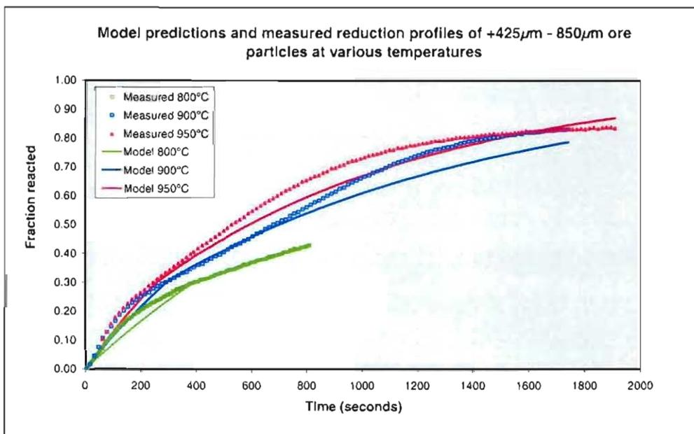
**Figure D 9:** Calculated (model) predictions and measured values regarding fraction of reducible oxygen removed as a function of time for ore particles in the size range -850 $\mu\text{m}$  +425 $\mu\text{m}$ .
