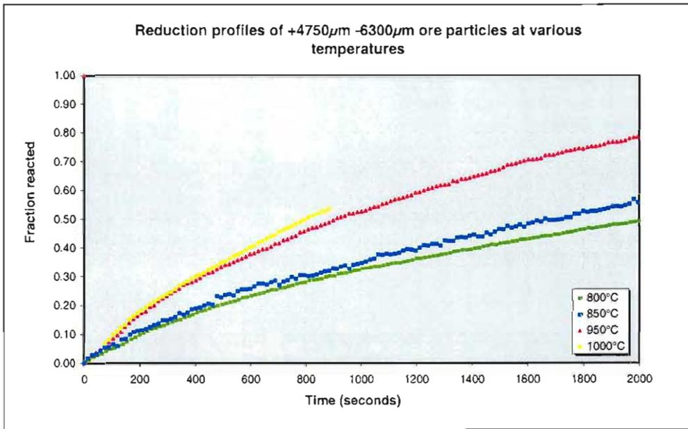
**Figure D 6:** Fraction of reducible oxygen removed as a function of reaction time during reduction of Sishen ore particles (in the size range  $-6300\mu\text{m} +4750\mu\text{m}$ ) with CO gas.
