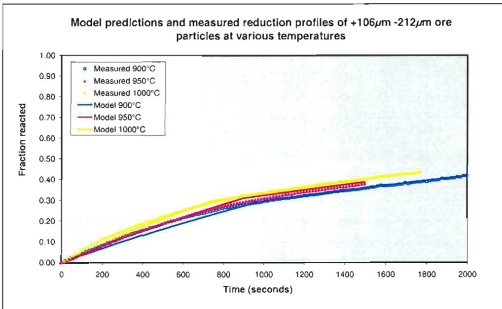
**Figure D 7:** Calculated (model) predictions and measured values regarding fraction of reducible oxygen removed as a function of time for ore particles in the size range  $-212\mu\text{m}$   $+106\mu\text{m}$ .
