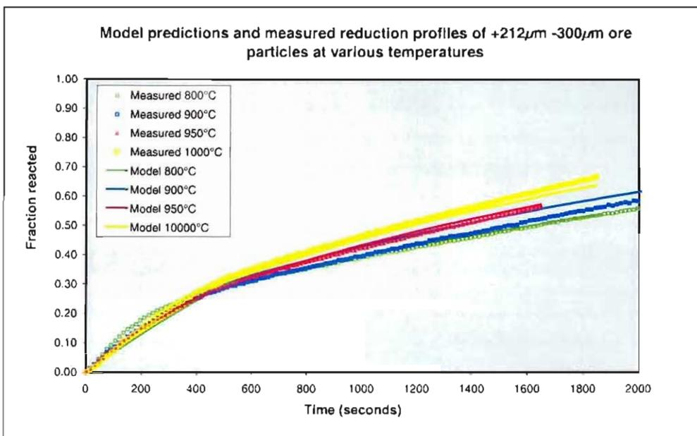
**Figure D 8:** Calculated (model) predictions and measured values regarding fraction of reducible oxygen removed as a function of time for ore particles in the size range -300 $\mu\text{m}$  +212 $\mu\text{m}$ .
