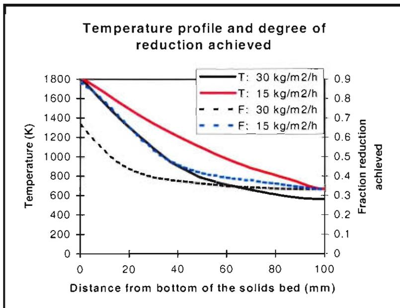
**Figure E 10:** Theoretical profiles of temperature and fraction reduction achieved through a 100mm high solids bed, for a production rate of 30kg/m<sup>2</sup>/h as well as 15kg/m<sup>2</sup>/h.
