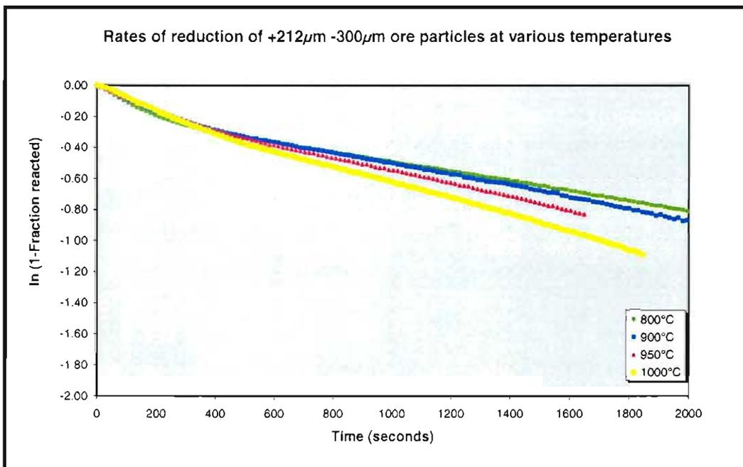
**Figure D 3:** *ln (1-Fraction of reducible oxygen removed) as a function of reaction time during reduction of Sishen ore particles (in the size range -300 $\mu$ m +212 $\mu$ m) with CO gas.*
