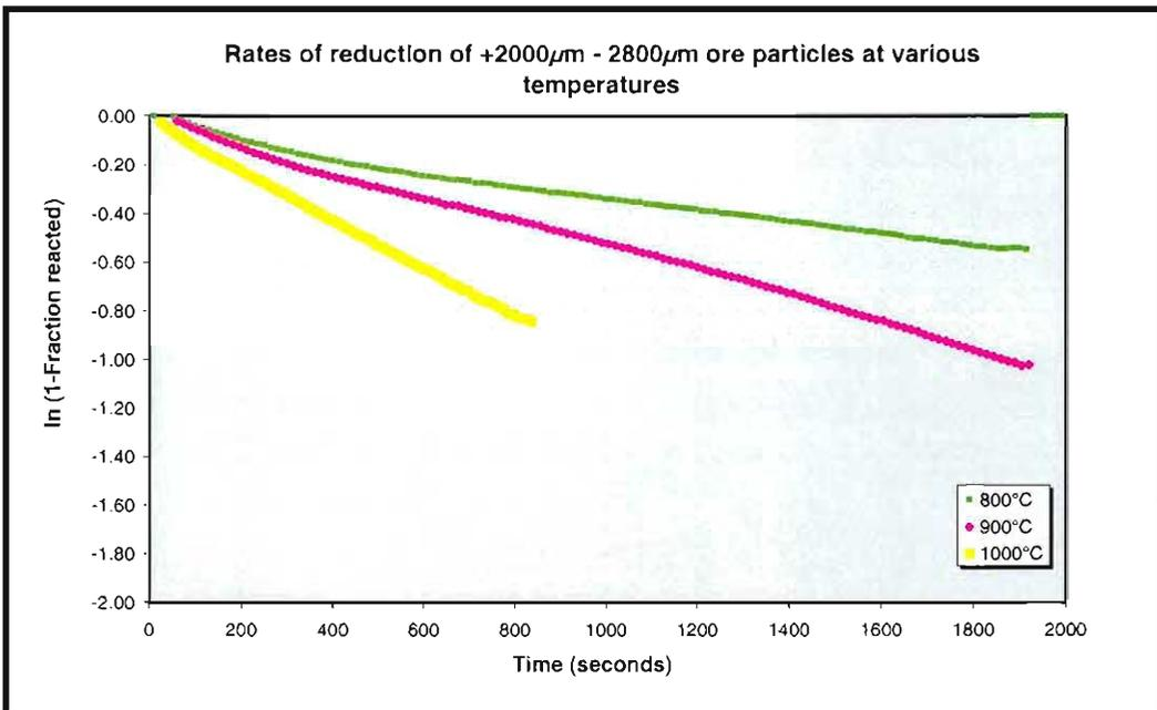
**Figure D 5:**  $\ln(1 - \text{Fraction of reducible oxygen removed})$  as a function of reaction time during reduction of Sishen ore particles (in the size range  $-2800\mu\text{m} +2000\mu\text{m}$ ) with CO gas.
