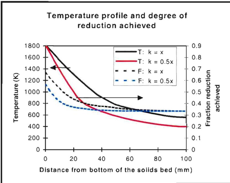
**Figure E 6:** Theoretical profiles of temperature and fraction reduction achieved through a 100mm high solids bed, for a production rate of 30kg/m<sup>2</sup>/h, when halving the thermal conductivity of the solids bed.
