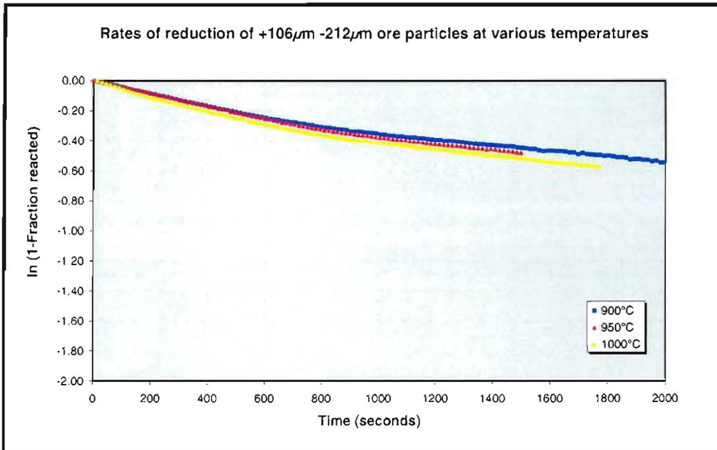
**Figure D 2:** *ln (1-Fraction of reducible oxygen removed) as a function of reaction time during reduction of Sishen ore particles (in the size range -212 $\mu$ m +106 $\mu$ m) with CO gas.*
