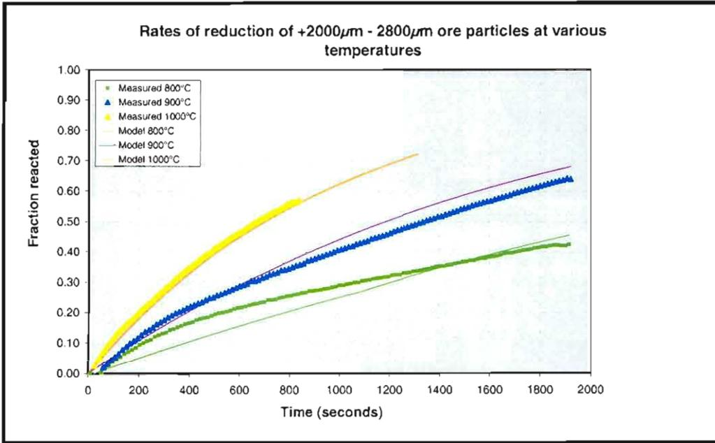
**Figure D 10:** Calculated (model) predictions and measured values regarding fraction of reducible oxygen removed as a function of time for ore particles in the size range - 2800 $\mu\text{m}$  +2000 $\mu\text{m}$ .
