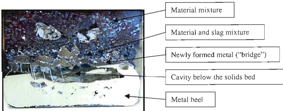
Figure F 4: Visual image of an impregnated cross section of a sample
