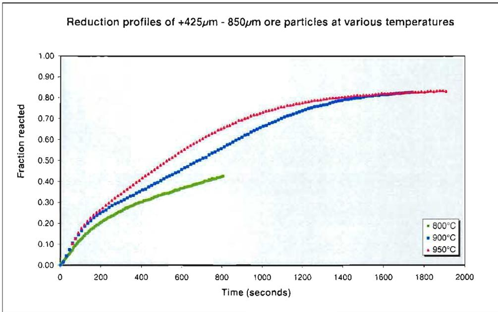
**Figure D 4:** Fraction of reducible oxygen removed as a function of reaction time during reduction of Sishen ore particles (in the size range  $-850\mu\text{m} +425\mu\text{m}$ ) with CO gas.
