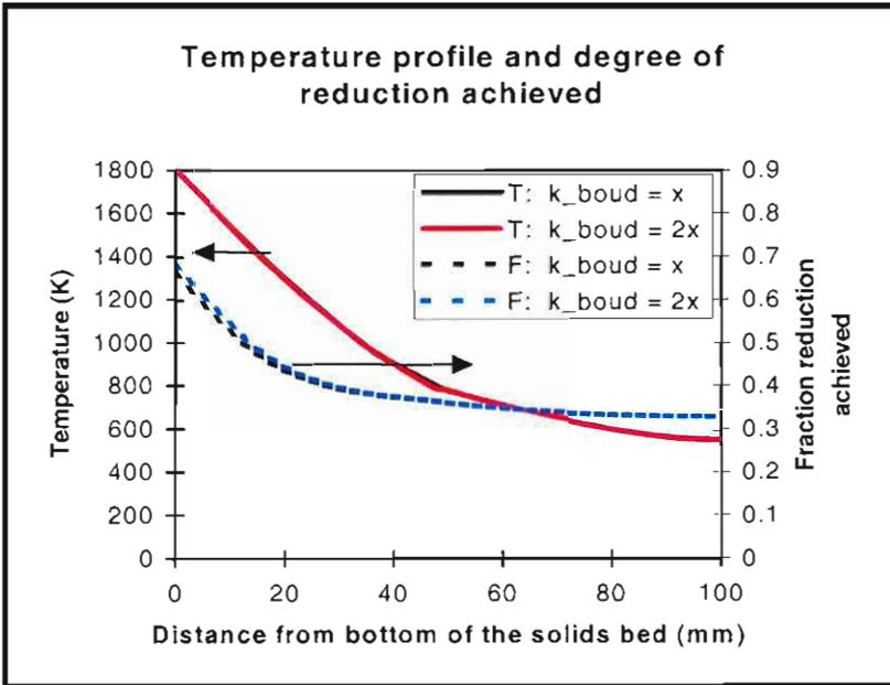
**Figure E 3:** Theoretical profiles of temperature and fraction reduction achieved through a 100mm high solids bed, for a production rate of  $30\text{kg}/\text{m}^2/\text{h}$ , when doubling the rate constant for the gasification reaction.
