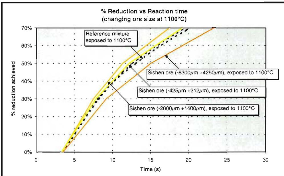
**Figure C 10:** Reduction rate of base mixture and a mixture containing various size fractions of Sishen ore during exposure to 1100°C.
