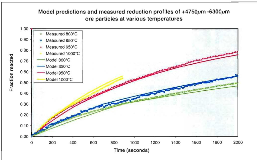
**Figure D11:** Calculated (model) predictions and measured values regarding fraction of reducible oxygen removed as a function of time for ore particles in the size range - 6300 $\mu\text{m}$  +4750 $\mu\text{m}$ .
