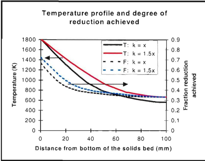
**Figure E 5:** Theoretical profiles of temperature and fraction reduction achieved through a 100mm high solids bed, for a production rate of 30kg/m<sup>2</sup>/h, when increasing the thermal conductivity of the solids bed 1.5 times.
