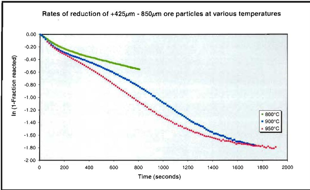
**Figure D 4:**  $\ln(1 - \text{Fraction of reducible oxygen removed})$  as a function of reaction time during reduction of Sishen ore particles (in the size range  $-850\mu\text{m} +425\mu\text{m}$ ) with CO gas.
