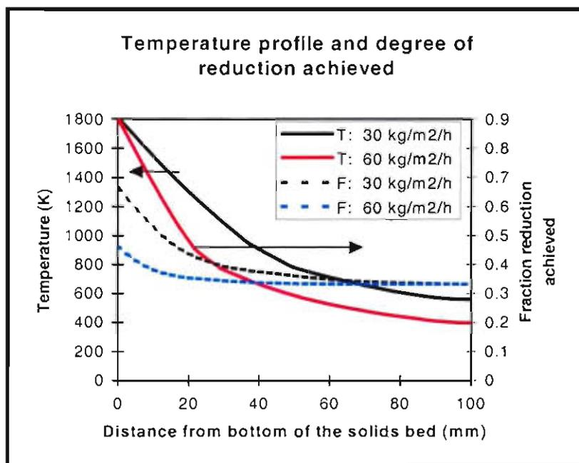
**Figure E 9:** Theoretical profiles of temperature and fraction reduction achieved through a 100mm high solids bed, for a production rate of 30kg/m<sup>2</sup>/h as well as 60kg/m<sup>2</sup>/h.
