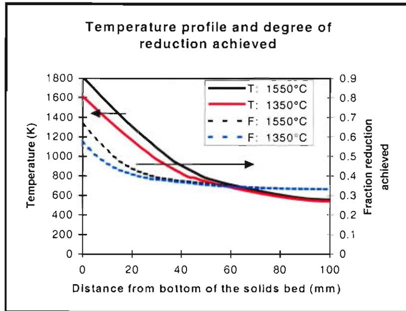
**Figure E 8:** Theoretical profiles of temperature and fraction reduction achieved through a 100mm high solids bed, for a production rate of 30kg/m<sup>2</sup>/h, decreasing the bath temperature from 1550°C to 1350°C.
