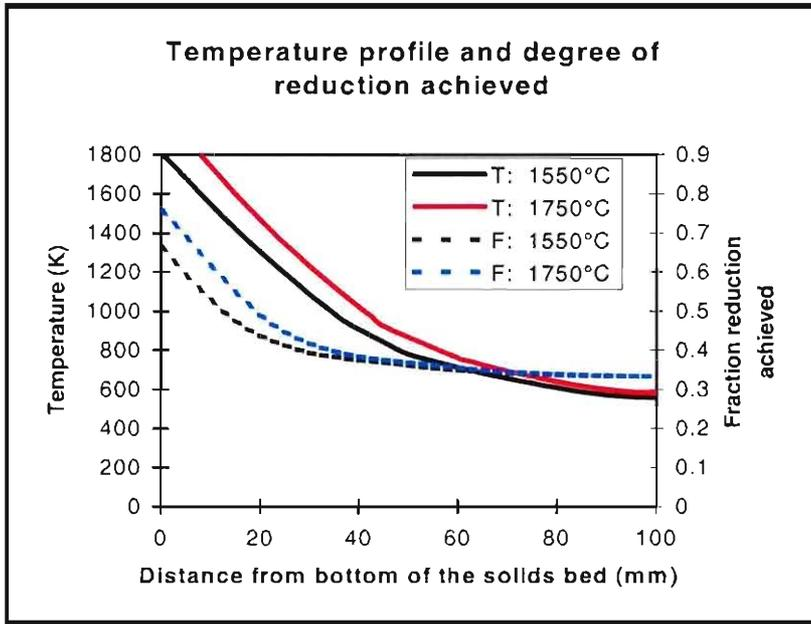
**Figure E 7:** Theoretical profiles of temperature and fraction reduction achieved through a 100mm high solids bed, for a production rate of 30kg/m<sup>2</sup>/h, when increasing the bath temperature from 1550°C to 1650°C.
