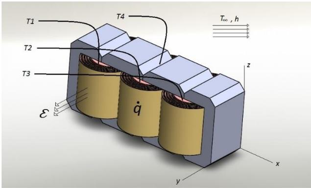
**Figure 1** Thermal model of the core.
