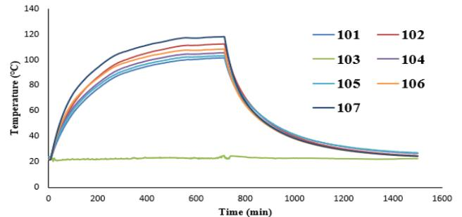
Figure 9 Temporal evolutions of the experimental temperatures in the transformer with linear load.
