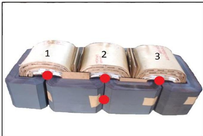
Figure 7 Position of Temperature Sensors
