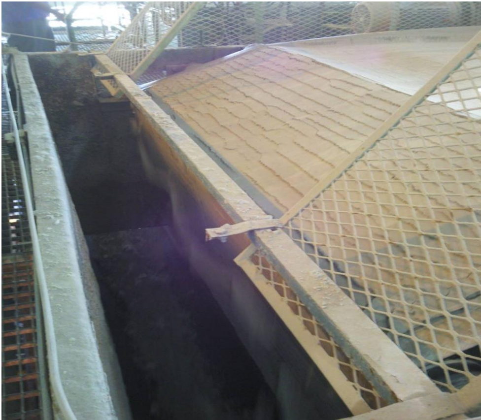
Figure 6: Horizontal belt filter discharge of filtered cake
