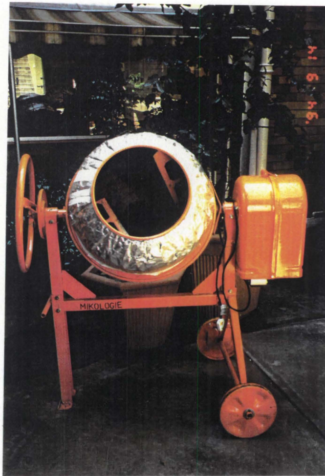
Figure 20 Converted cement mixer used at the University of Pretoria to produce a good blend of casing medium and neutralizing agent for pasteurization.
