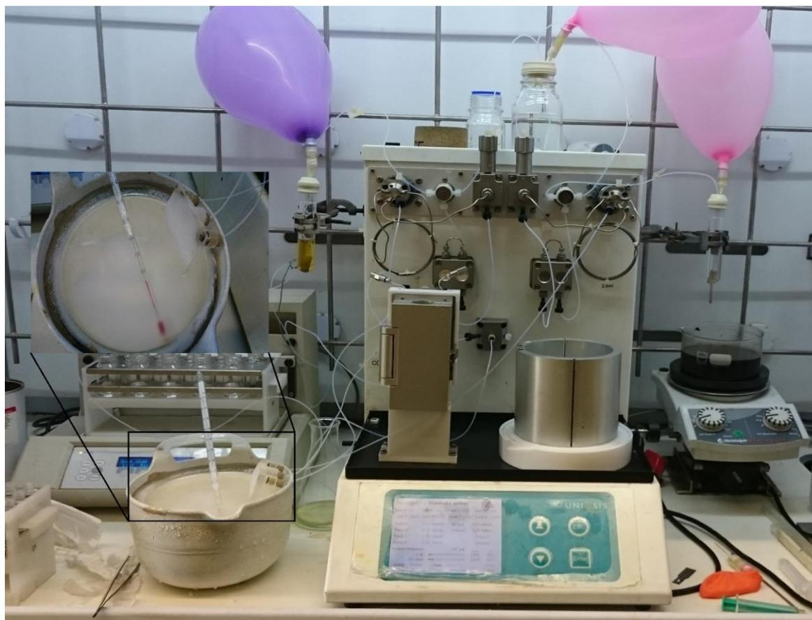
**Figure 6.5.** Stage 2A stand-alone setup with the mixing chip in the cold-bath at -82 °C.
