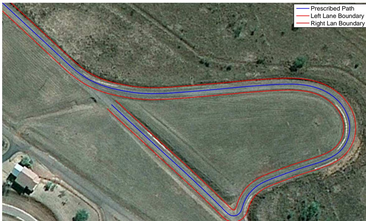
Figure 6.22: Satellite image of Gerotek dynamic handling track top section with lane boundaries (Gerotek, 2011a).
