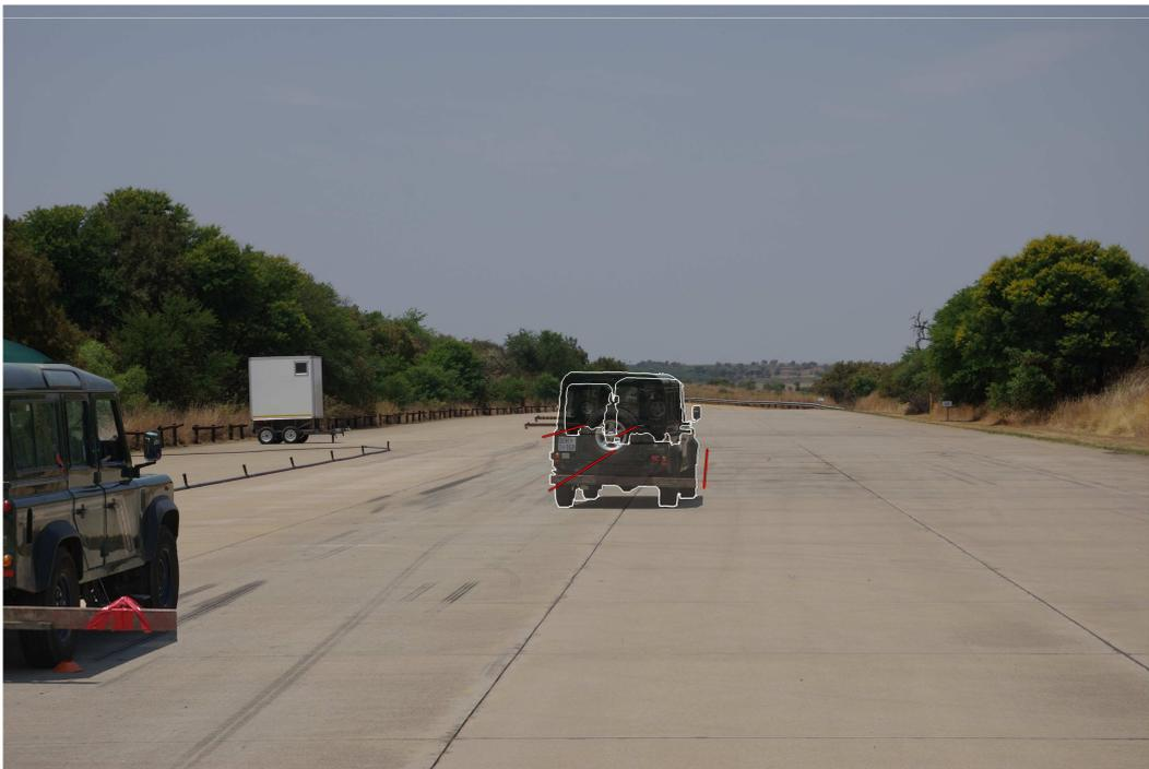
Figure 6.9: Vehicle following path through DLC at 40km/h.
