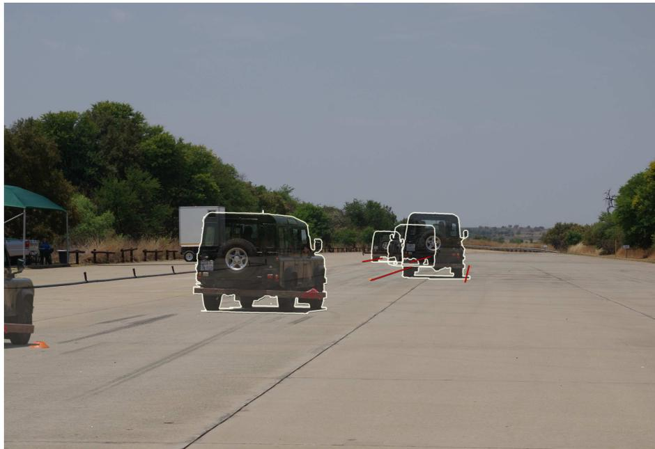
Figure 6.5: Vehicle following path through DLC at 20km/h.
