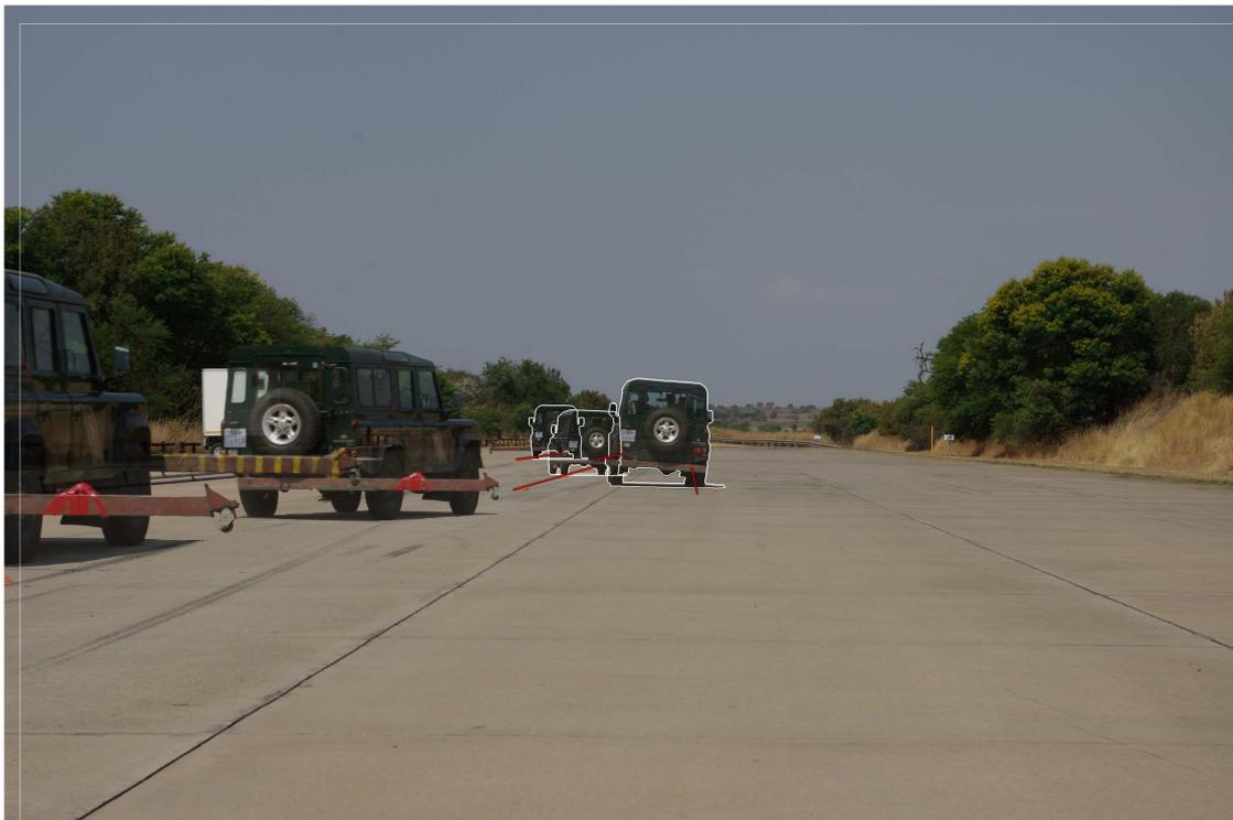
Figure 6.19: Vehicle following path through DLC at 80km/h.
