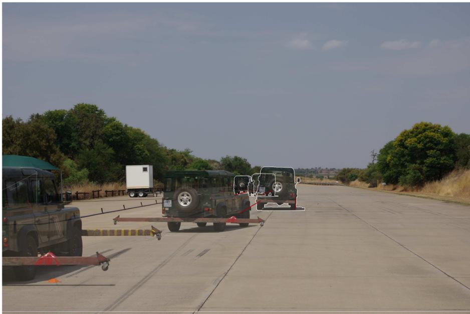
Figure 6.13: Vehicle following path through DLC at 60km/h.
