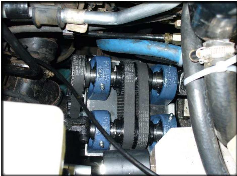
Figure 2.5: Stepper motor assembly installed in engine bay.
