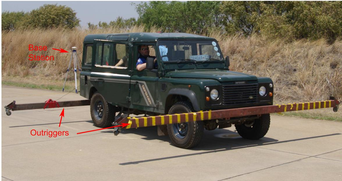
Figure 6.1: Test vehicle equipped with outriggers to prevent rollover.
