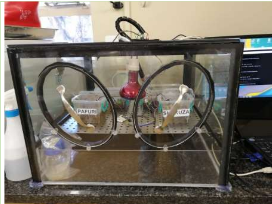
Figure 9: The developed terra-simulator holding the individual soil containers along with the soil, light and humidity sensors.
