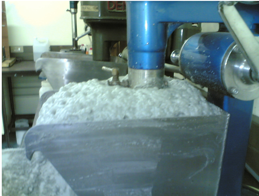
Figure 5.7: Picture of the 8-litre flotation cell with talc being floated using Dowfroth 200 frother.
