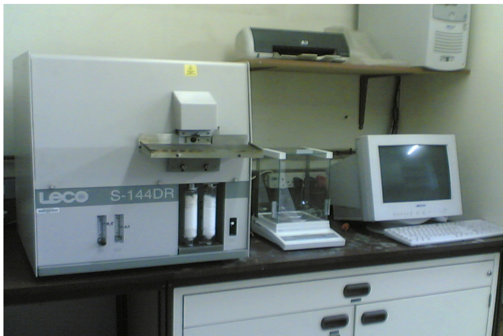
Figure 3.4: Picture of the sulphur analyzer machine that was used for sulphur analysis
