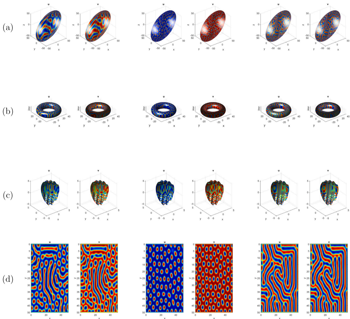
Fig. 6. Spatiotemporal distributions showing some Turing patterns on different surfaces for Gray-Scott model. Plots (a-d) correspond to sphere-, torus-, bumpy- and plane- surfaces, respectively. While columns 1–3 stands for evolution of spots/strips, spots and stripes patterns, respectively.
