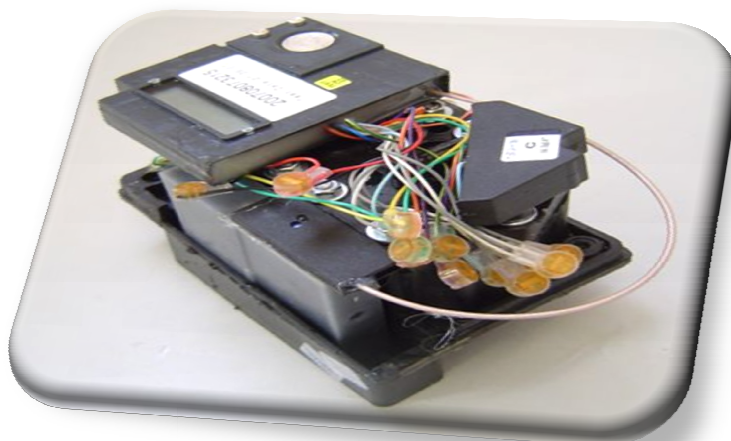
Figure 20: The electronic part of the meter with the many scotch locks on the ends of the wires
