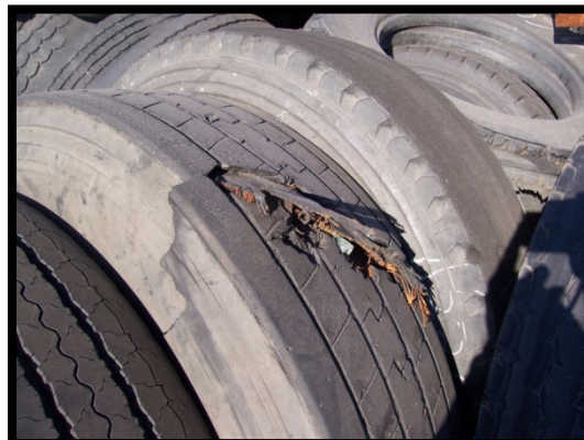
Figure 13 : Tyre damage due to impact on bad roads
