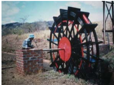
Left: Illus 9.11: Example of a coil waterwheel used in Zimbabwe. ( http://aquamor.tripod.com/Wheel.htm )
