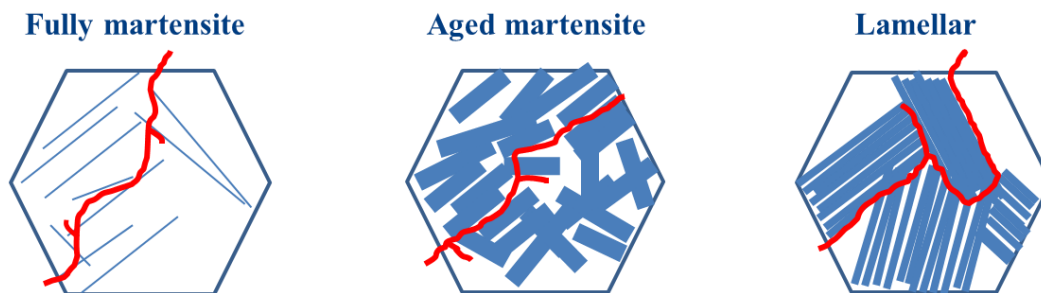
Figure 5.1: A schematic diagram showing the difference in crack propagation through various microstructures of the Ti-6Al-4V alloy
