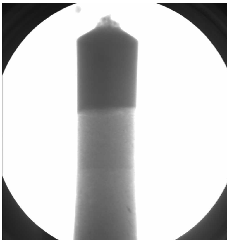
Figure 4.8: X-ray image of a misfire sample with 28% Al wt content
