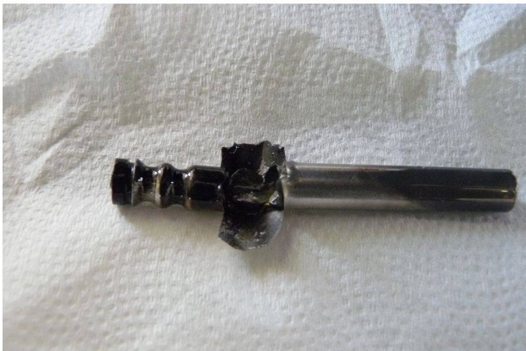
Figure 4.9: Destroyed detonator with aluminium Charlize element filled with thermite composition containing 20 wt % sensitiser
