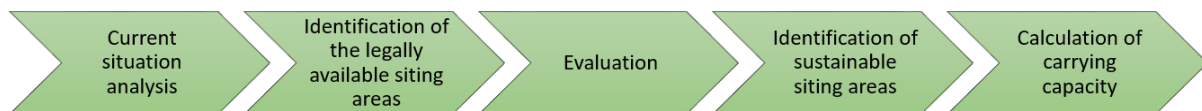
Figure 59: The workflow implemented by Tsoutsos et al. (2015) for regional wind farm planning.
