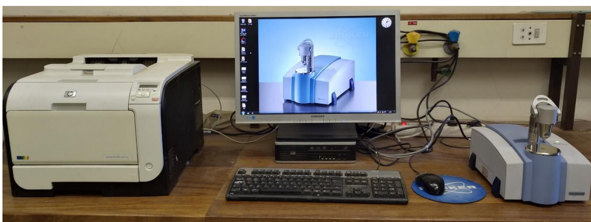
Figure 4.2: Bruker Alpha Platinum ATR
