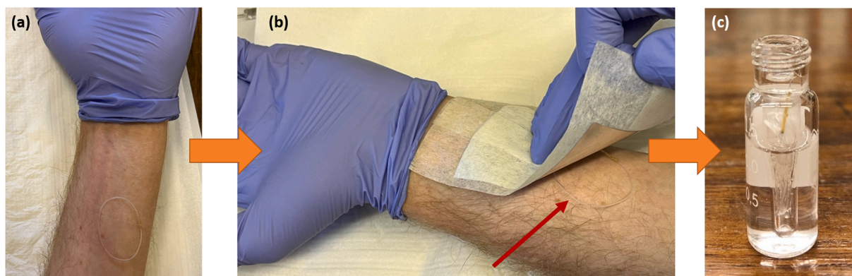
Fig. 1. Skin surface sampling procedure. (A) The ethanol modified PDMS sampler on the inner arm. (B) the Mylar® sheeting with medical adhesive tape securing the sampler. (C) Micro-solvent back extraction of the PDMS sampler in an LC vial insert.
