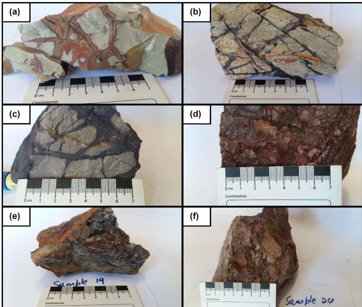
Figure 4.10:Schikloof Formation - (a, b & c) Hydrothermal crackle breccias with a >5mm clasts size and a matrix. These breccias generally have than 75% large clasts. (d, e & f) Hydrothermal mosaic to chaotic breccias where clasts have been partially or completely rotated. Roughly 50 to 65% of these rocks are made of clasts and the other 35 to 50% is the matrix.
