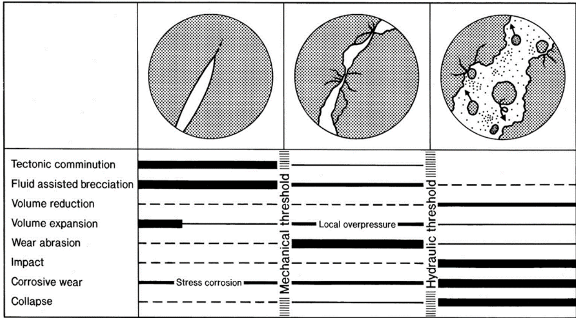
Figure 1.2: The three stages (propagation, wear and dilation) of hydrothermal breccia formation. These stages are separated by a mechanical discontinuity (between propagation and wear stages) as well as a hydraulic discontinuity (between wear and dilation); adopted from Jébrak (1997).
