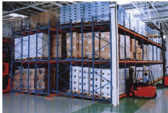
Figure 7: Push back racking system
