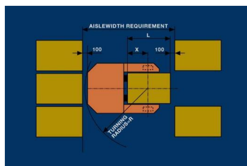
Figure 10: Reach truck aisle width application
