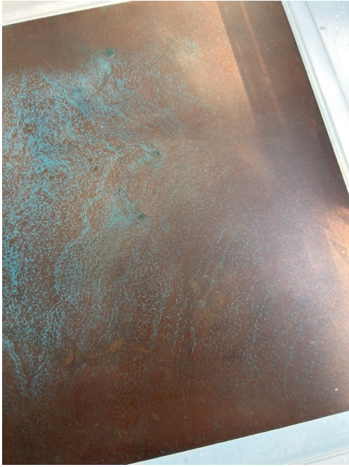
Figure 27: Detail of copper plate during oxidation (day 3), 12 August 2023.
