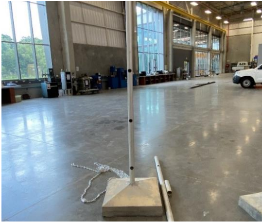
Figure A1. Aluminium pole with a concrete base for central water body temperature logging.
