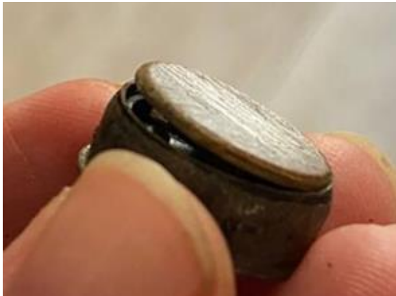
Figure A9. A faulty iButton that did not survive MD 2.5. The lid cracked open, and the Liquid Armour encapsulation was no longer present.
