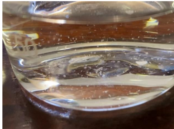
Figure A12. Precipitates in the final week of the assessment from the Liquid Armour beaker.
