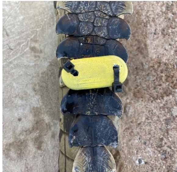
Figure A8. Liquid Armour encased 3D printed iButton.
