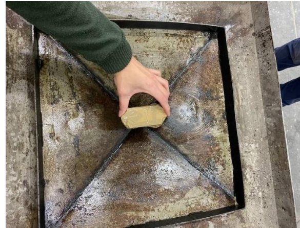
Figure A14. LHT65 LoRaWAN logger placement in the apex of the pyramid mould, prior to concrete addition.
