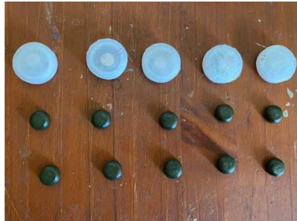
Figure A10. Liquid Armour (bottom) and 3D printed polypropylene (top) encapsulated batteries.
