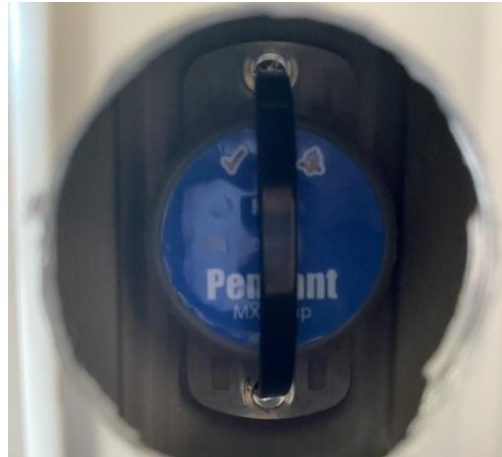
Figure A2. Holes drilled in the aluminium pole for Hobo pendant placement, secured by a cable tie.
