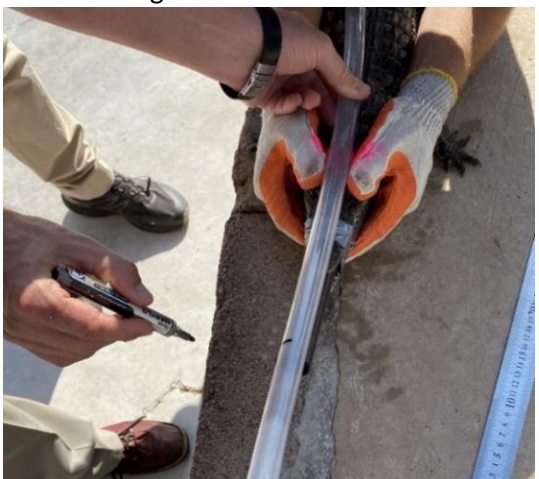
Figure A5. Measuring and marking the second piece of tubing, ensuring crocodile safety
