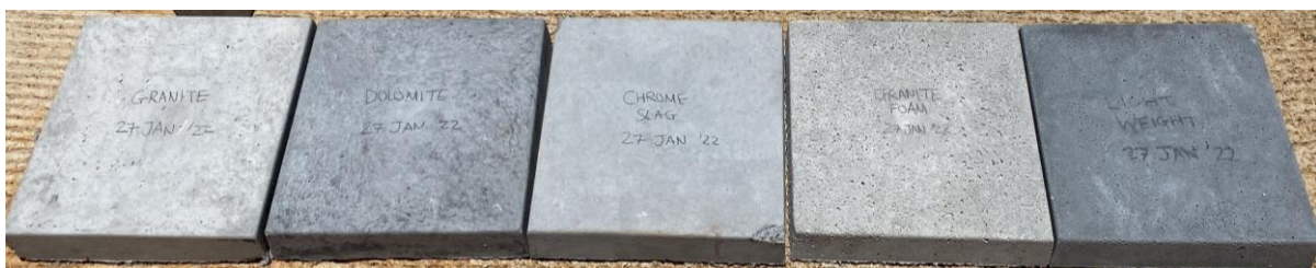
Figure 14. Concrete slabs from left to right: granite, dolomite, chrome slag, aerated granite, and lightweight dolomite.
