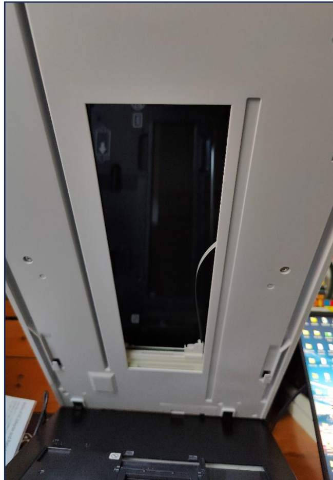
Figure 29: Transparency glass on Epson V600, to allow for the digitisation of negatives.
