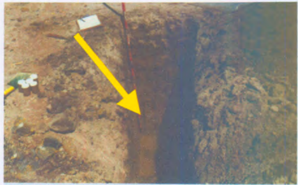
FIG. E.10 - Seepage in test pit C/2. A sample was taken for chemical analysis.
