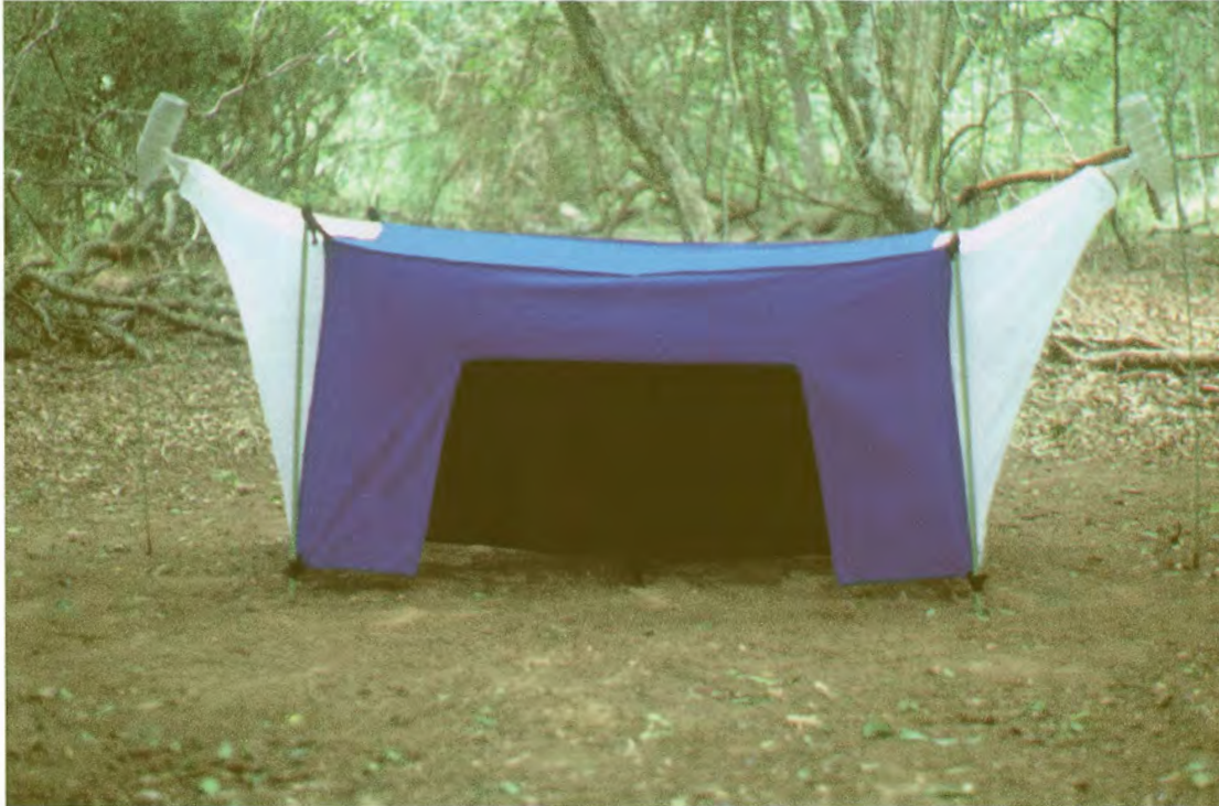
Fig. 4.3 Photograph of the final H trap design for the capture of G. brevivalpis and G. austeni (the trap is held upright by fastening the corners to four rigid metal poles (1,2 m long) and the cones are suspended from two flexible steel rods (1,4 m long))
