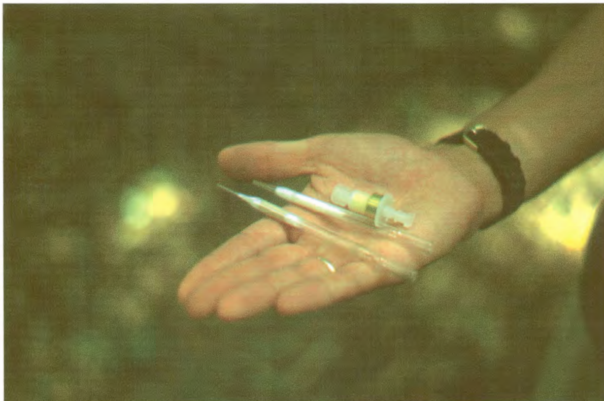
Fig. 3.3 b Collections of carboxylic acids were made by sampling through filters containing Chromasorb P AW filters (left), volatiles (i.e. phenols and octenol) were collected on Porapak® filters (centre) and ketones and aldehydes (carbonyl compounds) were trapped with silica SepPak® cartridges (right)
