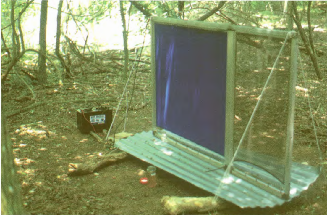
Fig. 2.1 Visual (1 x 1 m pthalogen blue) and non-visual (0,5 x 1 m net) electric grids incorporated to form a flanked target (i.e. p.blue/net).
