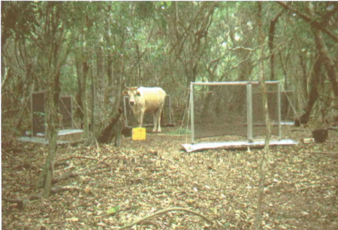
Fig. 6.1 Cow in the centre of an incomplete ring of six electric nets (8 m diam.) covering 35 % of the circumference of the ring
