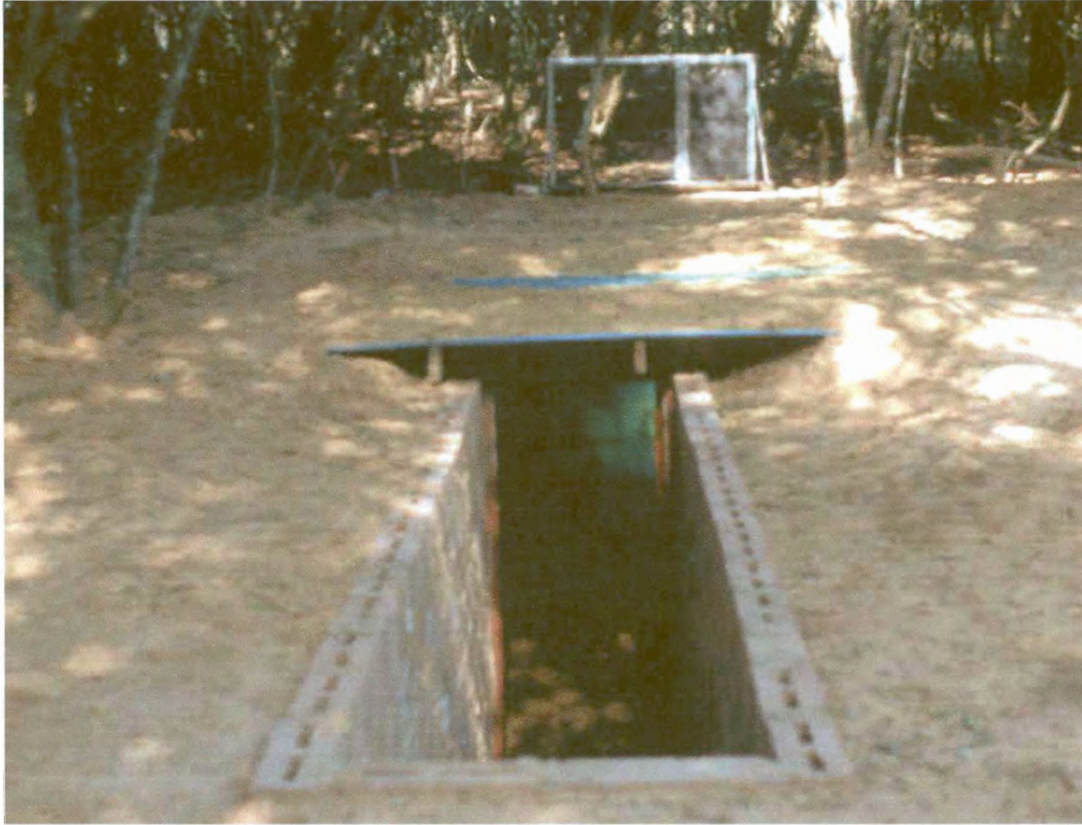
Fig. 3.4 Front view of ramp of pit. Setup shows 1,5 x 1 m electric net at far side of pit where ventilation shaft exits. Note fibre-glass sheet in roof of pit allowing light into pit
