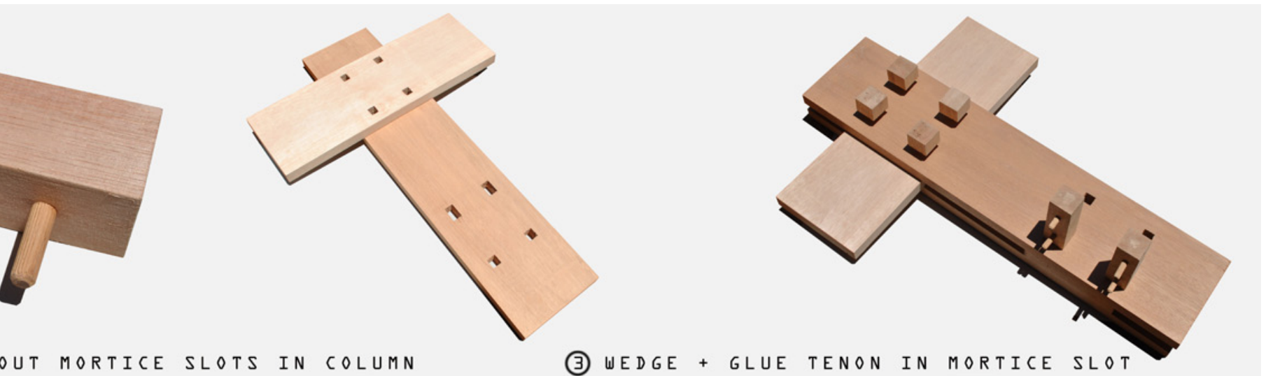
Fig. 7.22 Image showing the construction of the timber column and beam system. Image compiled by author (November 2012).
