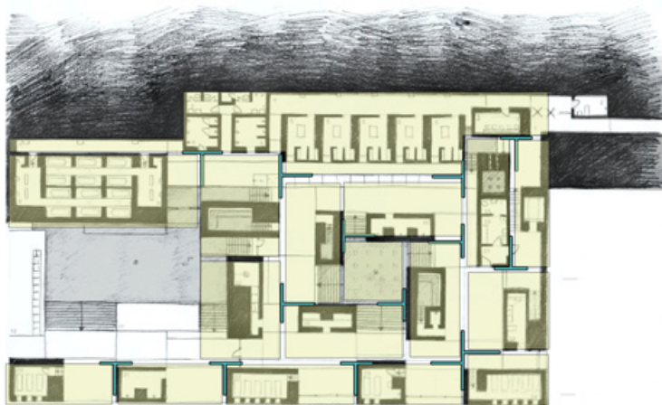
Fig. 5.12 Plan showing the different water temperatures and qualities of the baths. Illustration by author (August 2012) based on plan by Peter Zumthor Architects.
