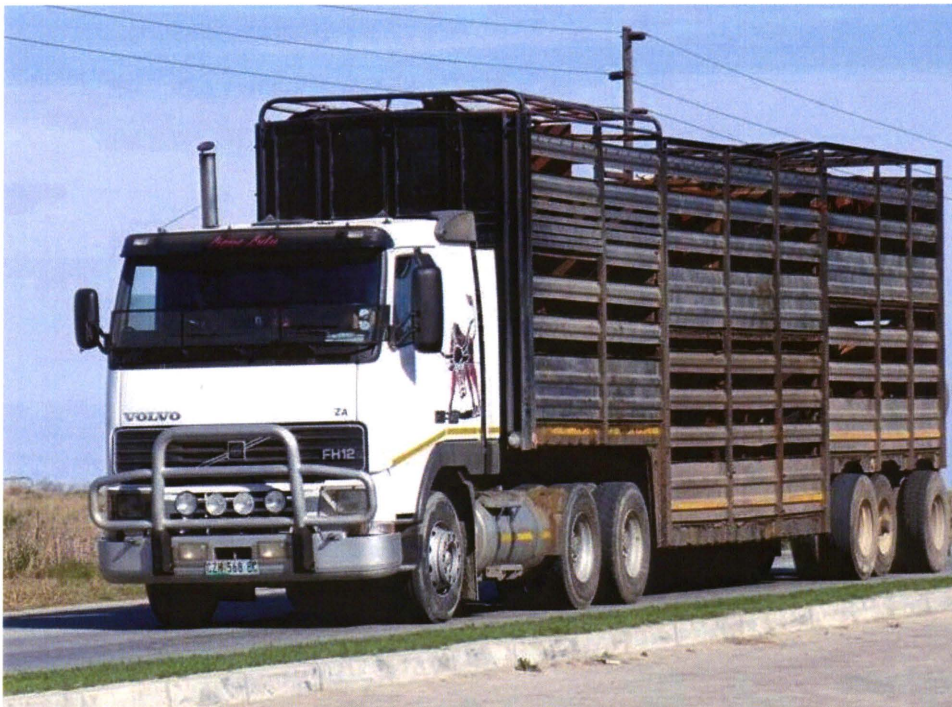
Figure 5.22 – Live cattle transport truck. Source: Own photograph
