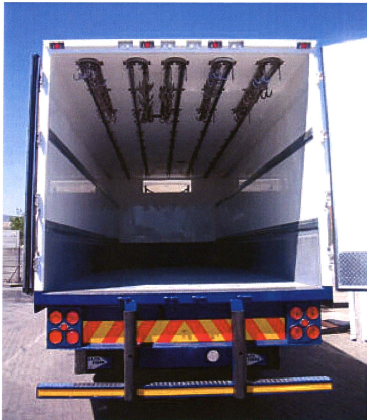
Figure 5.23 – Refrigerated delivery truck (with rail hangers), inside view. Source: Own photograph
