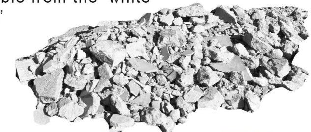
BUILDING RUBBLE FOR FOUNDATIONS AND AGGREGATE Found along all inward vehicular roads
