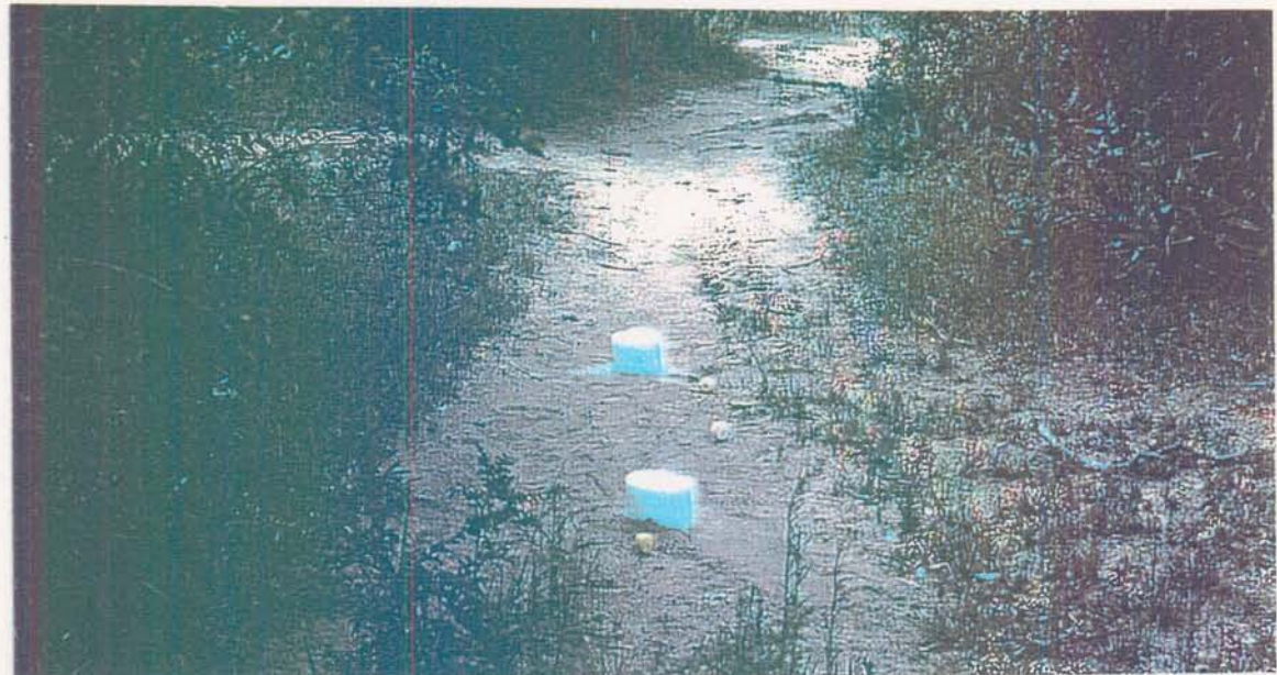
Fig. 17a) + b) The AAAP/CO 2 traps were easy to use in the field, and were often moved around. Six or more traps were used at a time (a), and the traps could be concentrated in sites where tick activity was highest (b).
