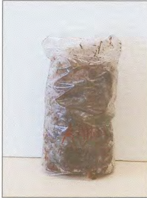
Figure 3.1: Completed plastic tubing reactor constructed for the biological pretreatment of Buffelsgrass.
