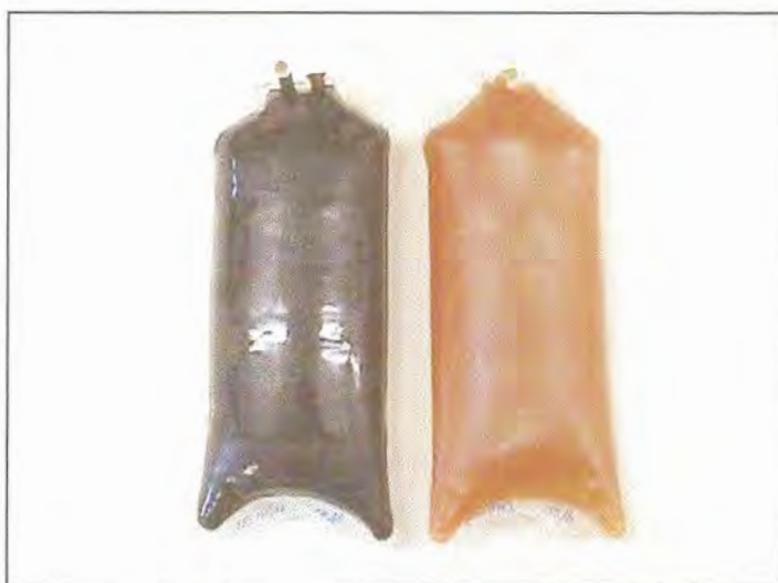
Figure 4.5: Comparison of the reactor that received 3% leachate (left) with the control reactor (right). Both reactors were inoculated with the inoculum produced in this study. Gas production was detected after 7 d in the leachate amended reactor, but not in the leachate-free control reactor.
