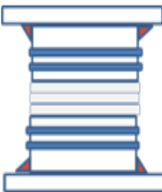
Welding of S/S convolution To Pipe End
