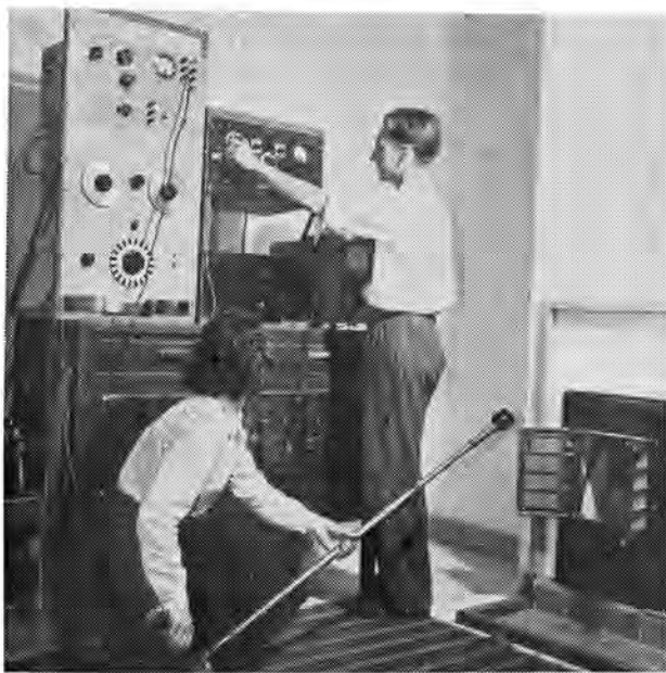
Electronic equipment being used to measure the amount of noise travelling through heating ducts.
