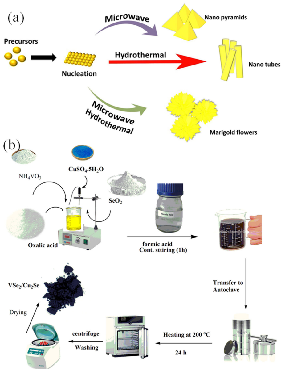
Figure 6. a) Schematic illustration of various morphologies in CdIn 2 S 4 . Reproduced with permission. [128] Copyright 2010, RSC. b) Synthetic route of VSe 2 @Cu 2 Se nanocomposites. Reproduced with permission. [129] Copyright 2023, Physica Scripta.
