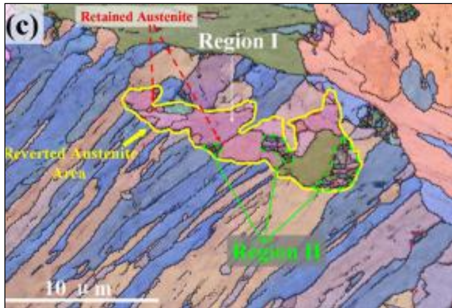
Figure 11: EBSD image of an interferritic region (You et al., 2013). Retained austenite refers to austenite that remains as such after solidification. Reverted austenite refers to austenite that underwent a transformation upon cooling. The sample is from a low-carbon HSLA steel that was reheated to simulate the HAZ region of a multipass weld.
