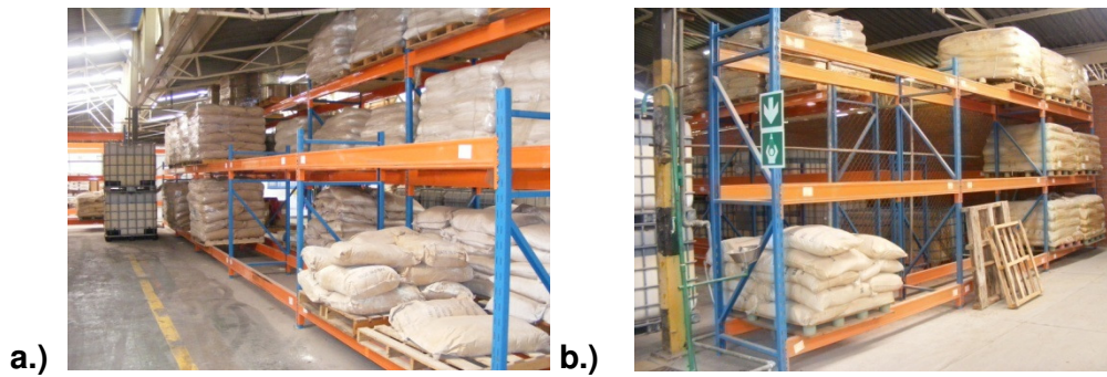
Figure 5-3: Pallet racks used at Simitri warehouse. a.) 3mX2.5mX1m. b.) 3mX4mX1m.
