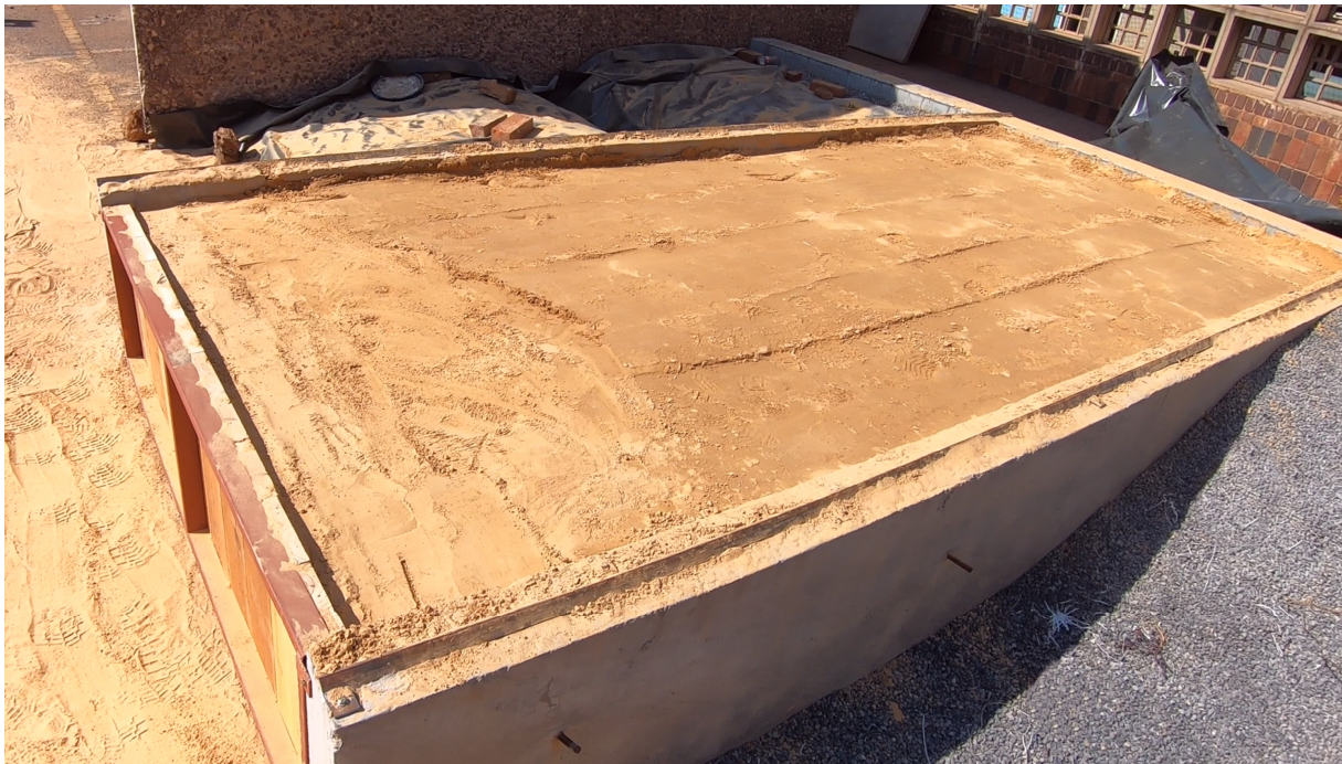
Figure 24-Soil bin commissioned at University of Pretoria (Length:5m, Breadth:2m, Depth:0.5m)
