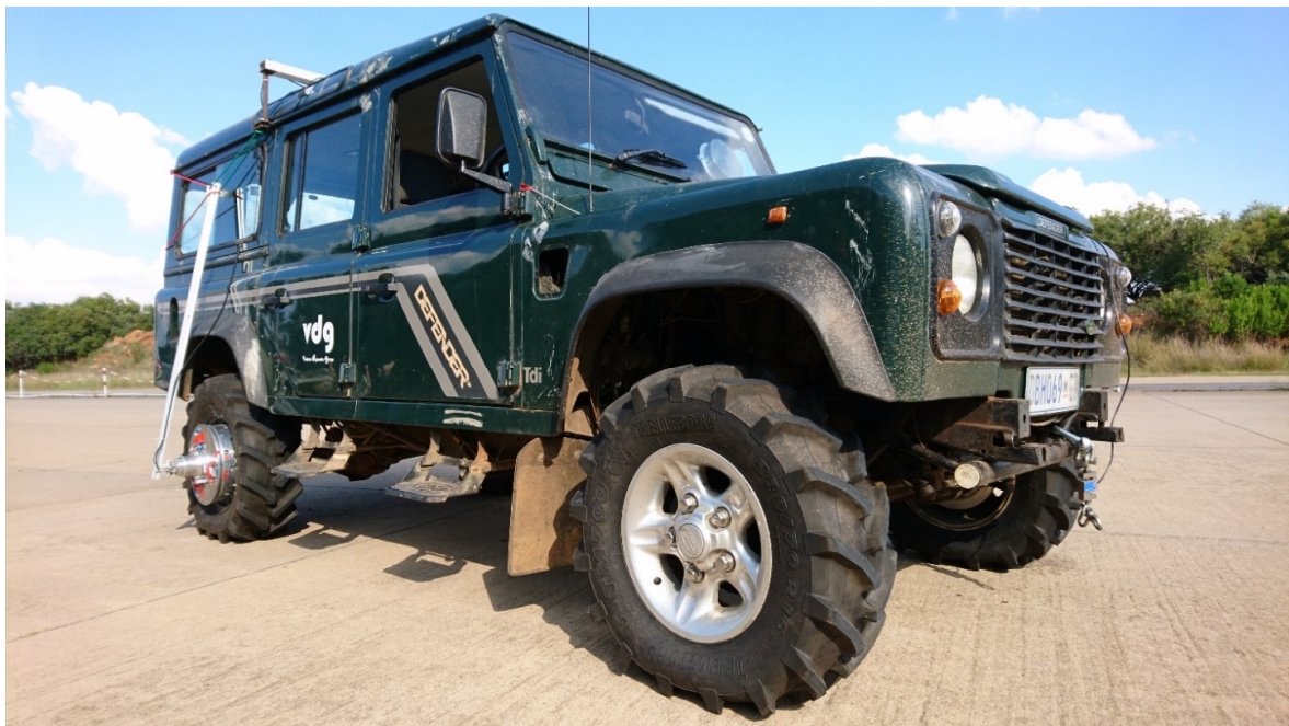
Figure 12-Target vehicle platform fitted with Trelleborg TM700-280/70R16 agricultural tyres (Becker, 2022).
