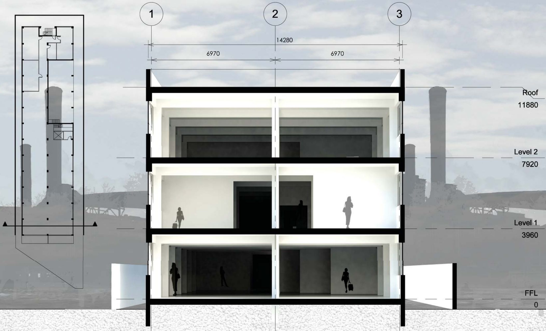
Fig. 3.7 Section through the building width, showing the basic dimensions of the structural grid
