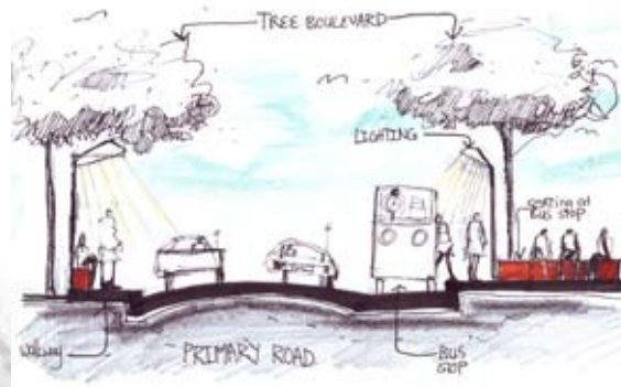
Fig. 7.4: Section A-A through the primary road with a tree boulevard, walkway, lighting, bus stop and seating areas (Author 2009).
