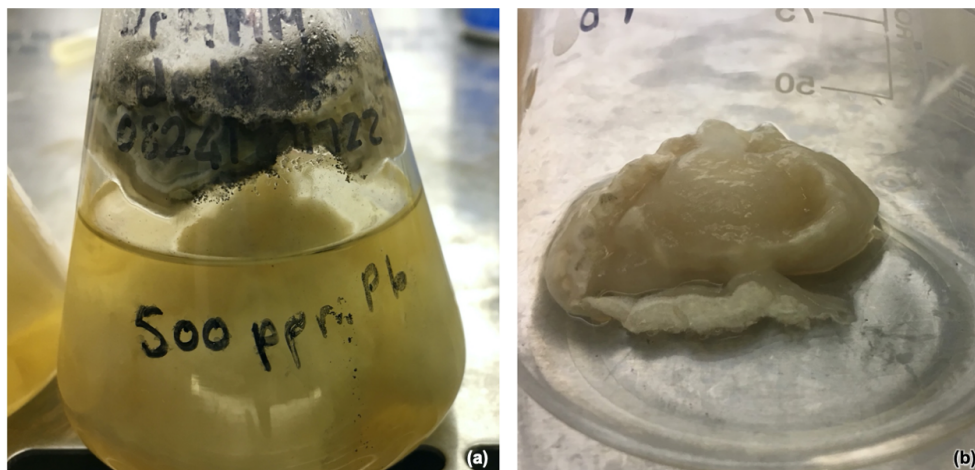
Figure 4.4: (a) Spores formed after three days where the mycelium came into contact with air, (b) Drained mycelium from a sacrificial sample after four days
