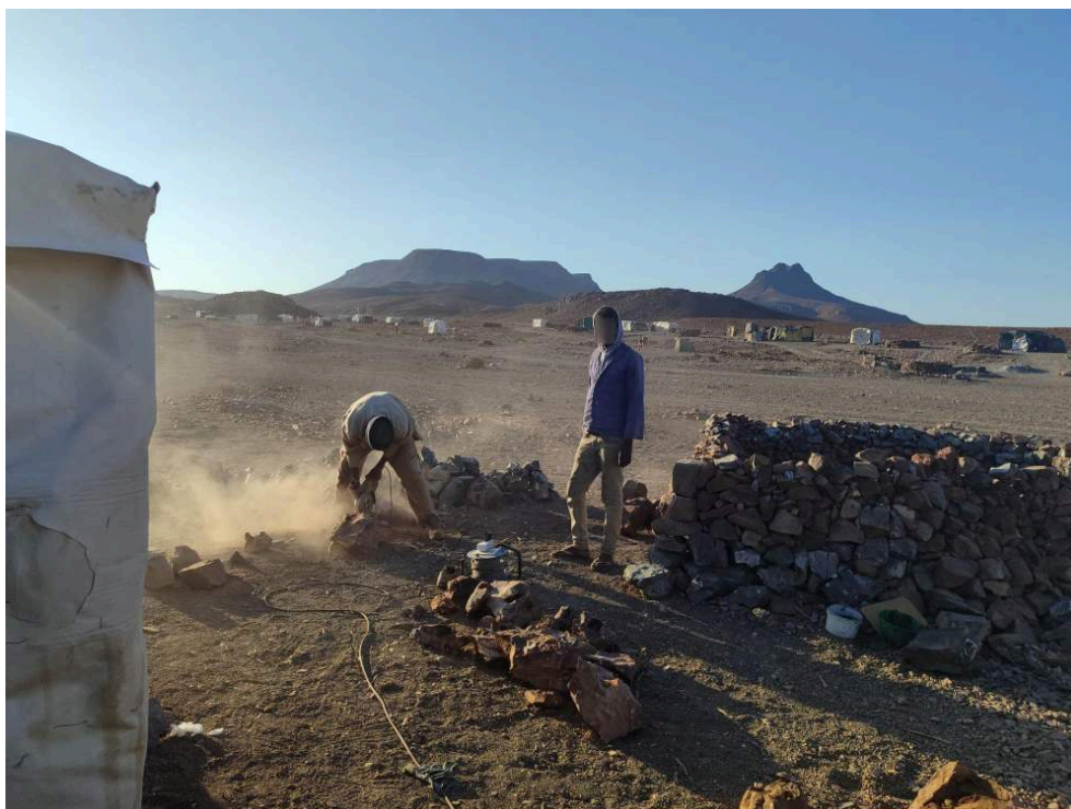
Figure 6: A daily life scene at Xoboxobos : Two miners take turns cutting a geode with an angle grinder
