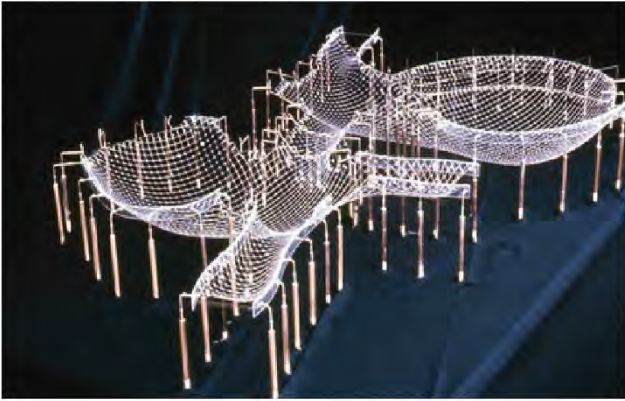
Figure 14: Final hanging chain model for Mannheim Multihalle (Liddell 2015: 41)
