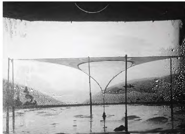
Figure 13: Physical model of a tensile roof by Frei Ott (Boller & Schwartz 2020: 570)
