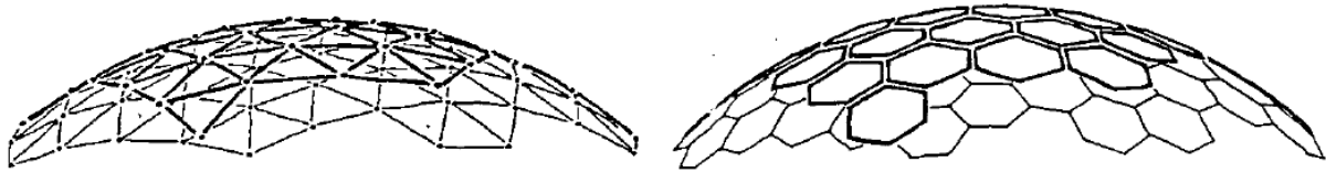
Figure 28: Triangular and hexagonal segmentation patterns for planar components based on the three-plate principle (Bagger 2010: 4)
