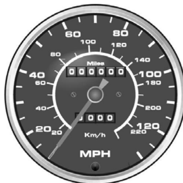
FIGURE 4 A speedometer that indicates ones speed in both kilometre and miles Source: http://www.g9toengineering.com/resources/reverseengineering.htm (2010/03/10)
