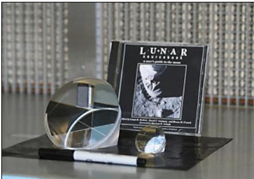
Figure 9: The fabricated 100 mm second generation retroreflector (left) placed next to the 38 mm Apollo retroreflector (right) of the first generation (source: Currie et al., 2011).
