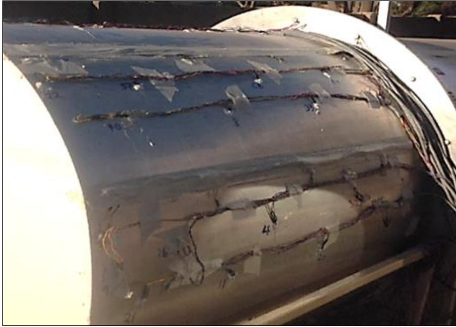
Figure 31: Thermally bonded RTD sensors for T_{\text{measured}} and T_{\text{reference}} on the test tube, all wired using the 12-core cat5e shielded cable. Visible strips/ patches of the insulation tape aided the alignment of the wiring.
