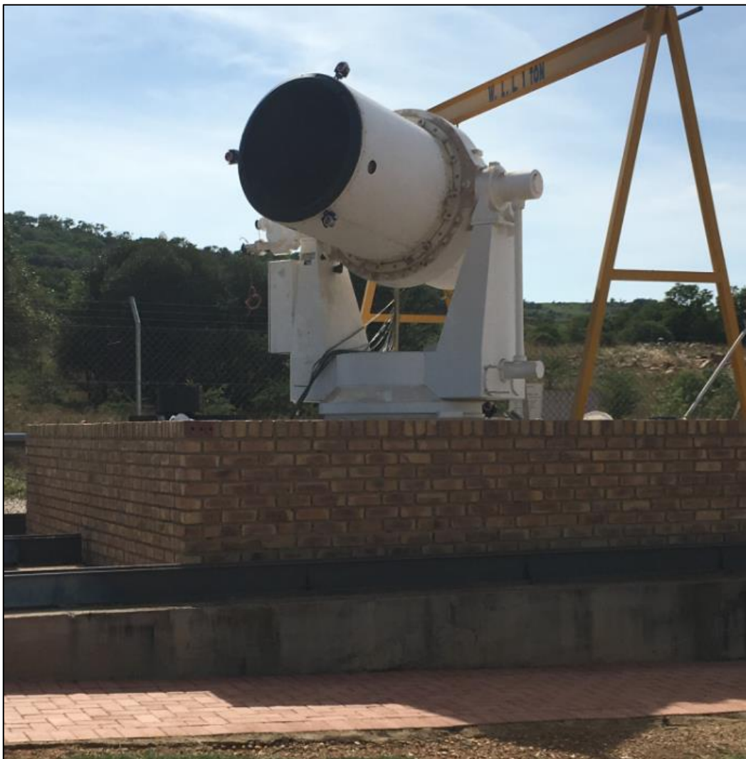
Figure 16: The ex-French 1-metre aperture Lunar Laser Ranging (LLR) stationed at Hartebeesthoek Radio Astronomy Observatory. The integration of other components such as the inner tube components is still in progress at HartRAO; hence are not shown.
