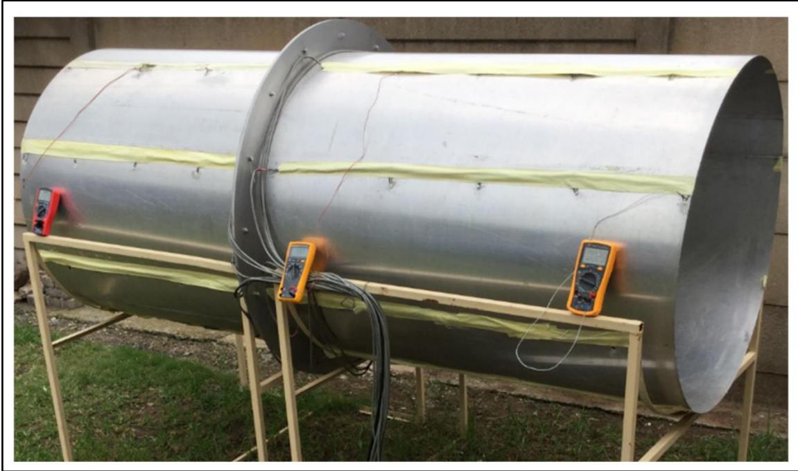
Figure 29: Troubleshooting and simple calibration setup of the tube showing the mounting and alignment of RTD sensors including the wiring and digital multimeters.
