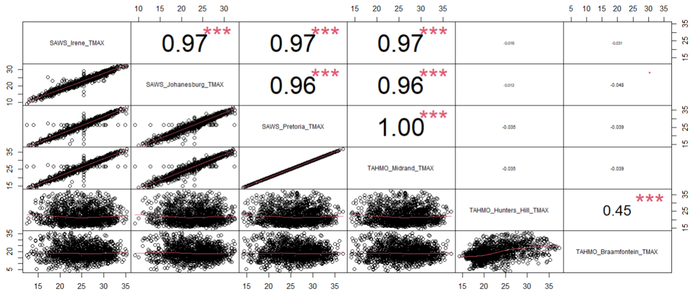
Figure 32: SAWS station vs TAHMO station showing significant correlation for temperature maximum (asterisk indicates significant correlation).
