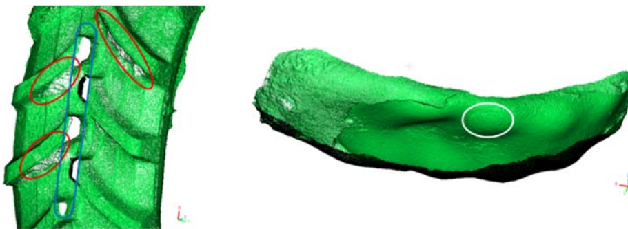
Figure 16. Poorly measured tread geometry highlighting missing sections of geometry (left) and poor reconstruction of measured inner surface showcasing different photogrammetry reconstruction problems (right)
