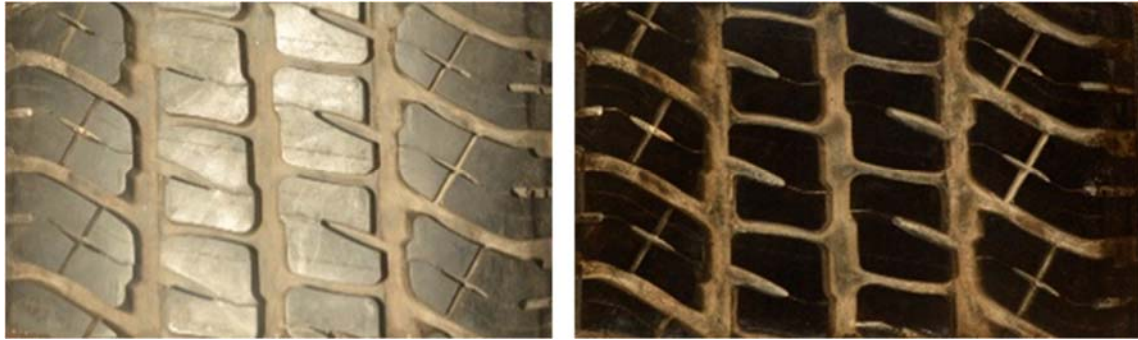
Figure 5. Effect of polarizing filters on reflections (Left - misaligned filters; Right - aligned filters) illustrating the evenly lit image resulting from the aligned polarizing filters.
