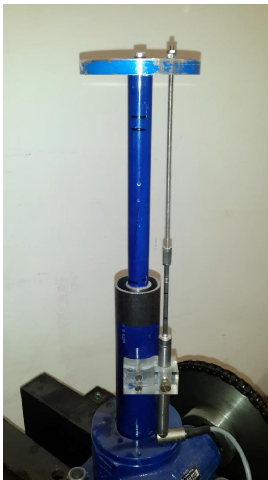
Figure 3.57: Close up of displacement transducer attached to jack
